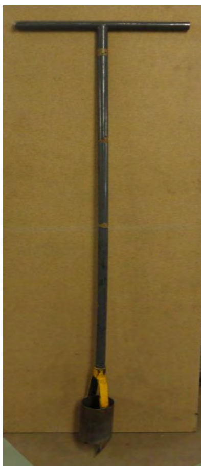
Figure 17: Photograph showing a soil auger. Photograph taken by Daniell (2013).
