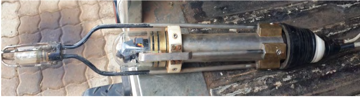
Figure 30: Down hole camera from the NWU used to conduct the down-hole camera survey. Photograph taken by Daniell (2014).
