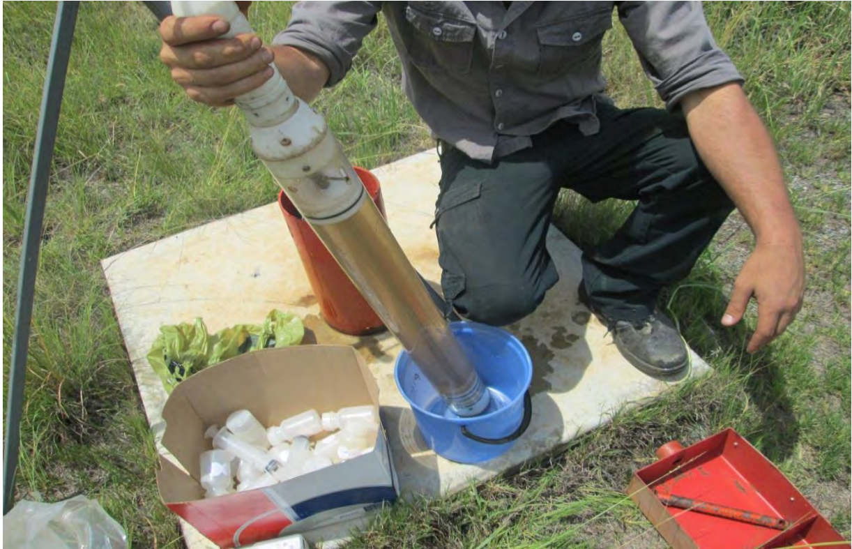
Figure 27: Photograph illustrating water being sampled with an electrical upgraded water sampler. Photograph taken by Daniell (2014).
