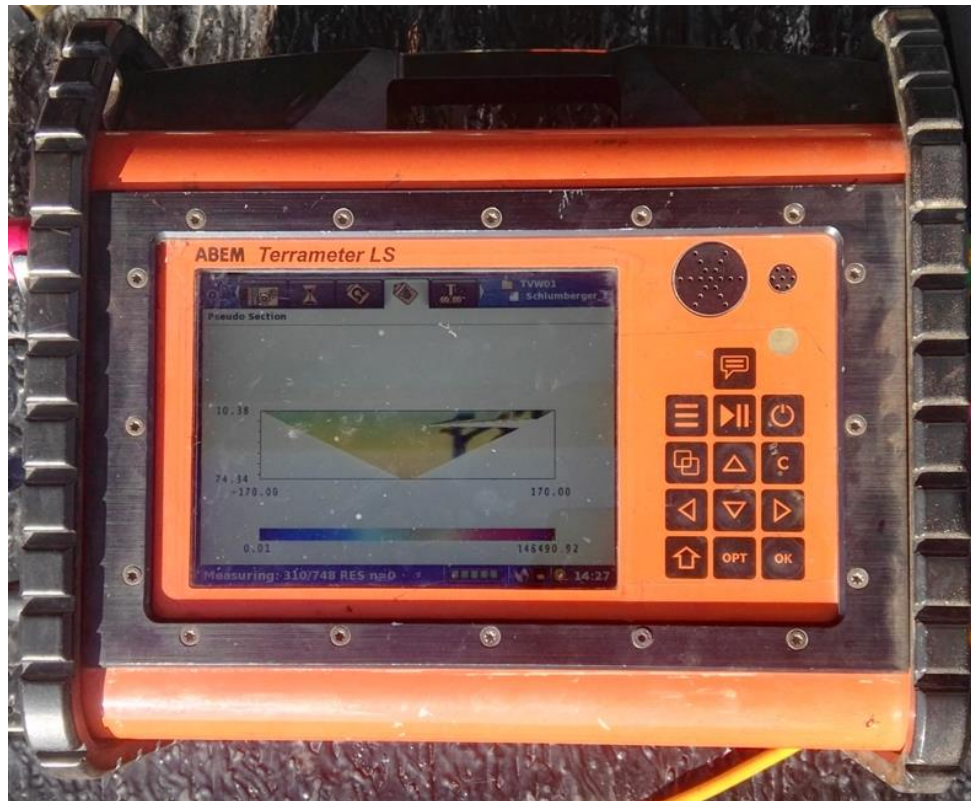
Figure 3-4: ABEM Terrameter LS 2 displaying a pseudo section while measuring during the fieldwork of this study. (T van Wyk, 2019)
