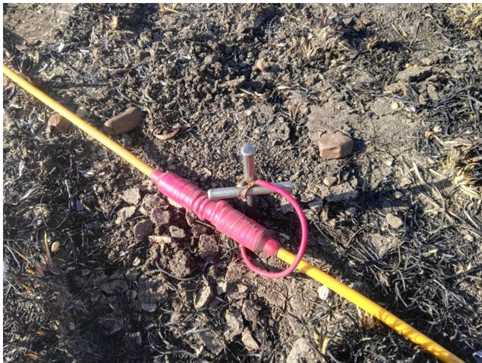
Figure 3-5: Stainless steel electrodes and cable connection during the fieldwork of this study. (T van Wyk, 2019).
