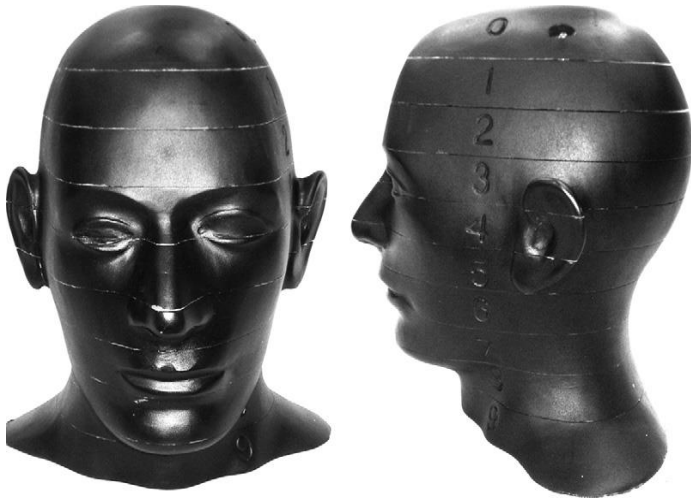
Figure 2: RANDO Phantom made with actual human bones embedded inside tissue simulating material (Palomo et al., 2008).
