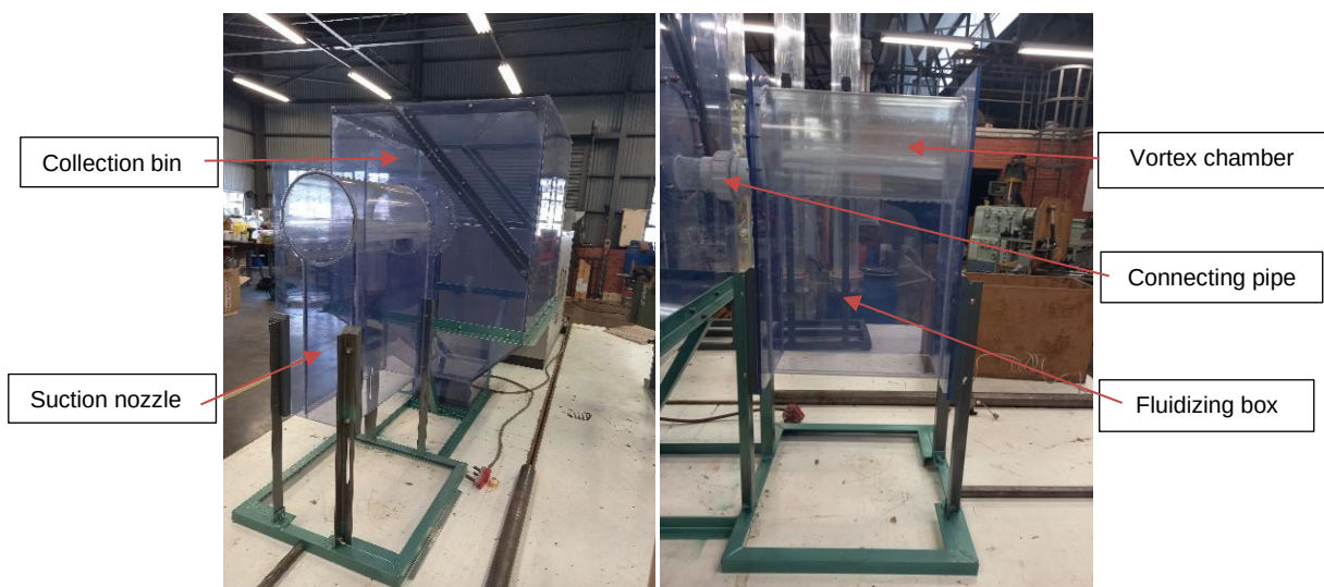
Figure 4.4: Images of the separating unit (left) and suction nozzle (right) including labelled sections.
