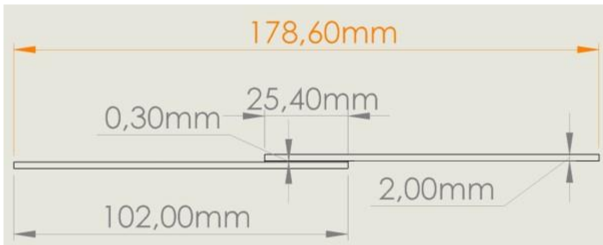
Figure 21: Joint sample geometry.
