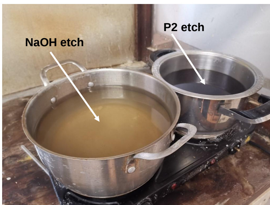
Figure 16: NaOH, left, and P2 etch, right
