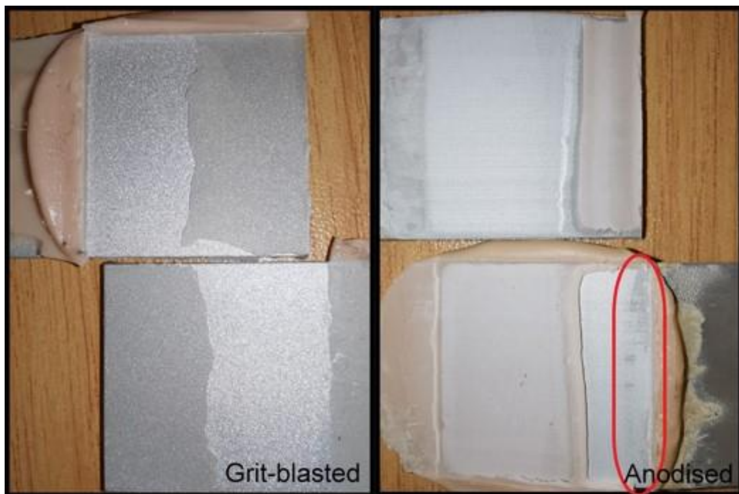
Figure 32: Fractured surfaces of unaged joints grit blasted and anodised
