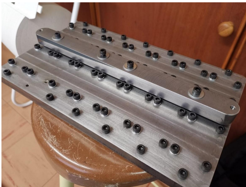
Figure 24: Adhesion alignment jig without any coupons
