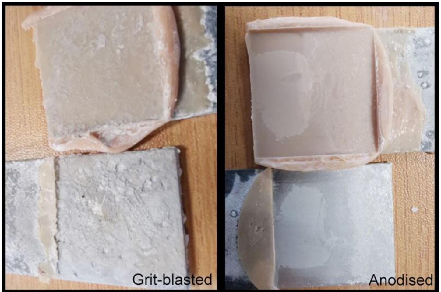
Figure 34: Fractured surfaces of 600 hours-aged joints.
