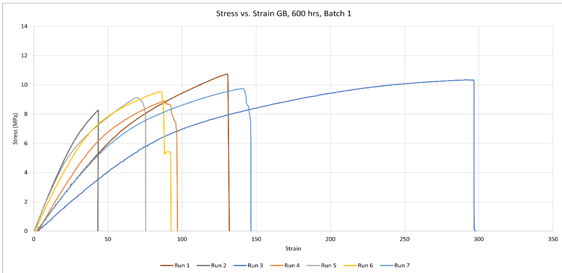
Figure 31 Stress vs. strain for grit blasted, 600 hours aged joints
