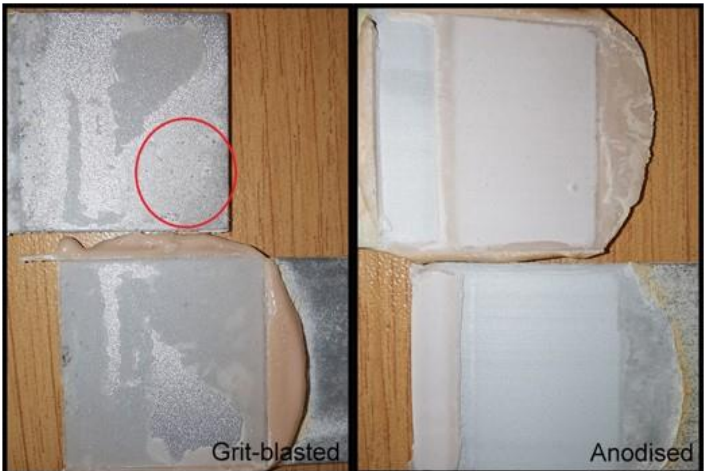
Figure 33: Fractured surfaces of 300 hours-aged joints.
