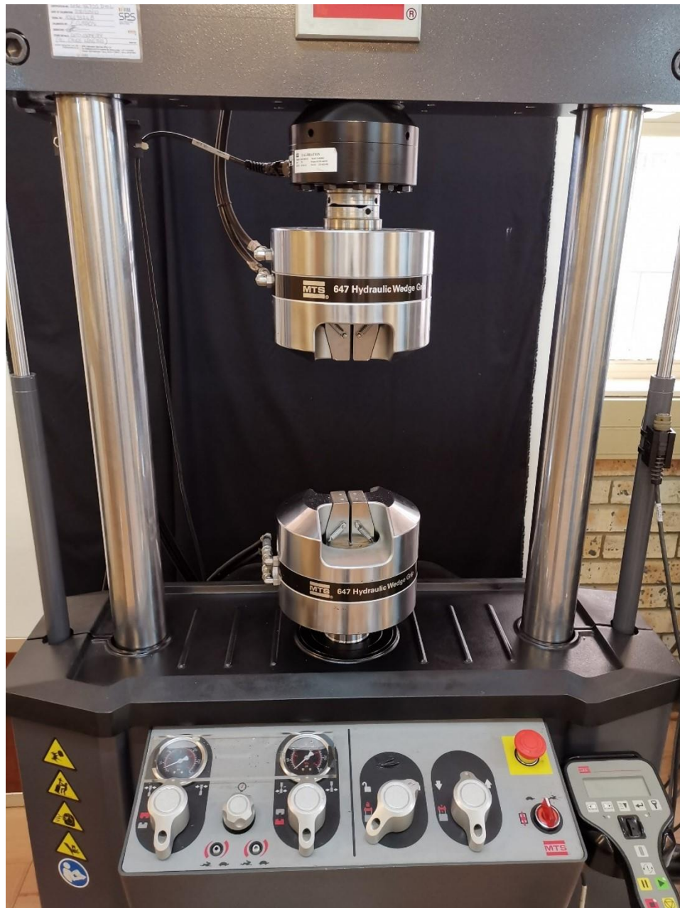
Figure 13: MTS Landmark Servohydraulic Testing System at NWU Materials Laboratory.
