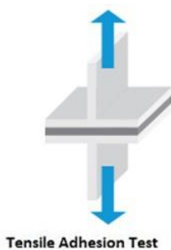
Figure 12: Schematic of tensile test (Saint-Gobain, 2020).
