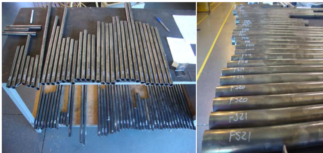
Figure 5-2: Photos of the individual pipes after being identified and cut
