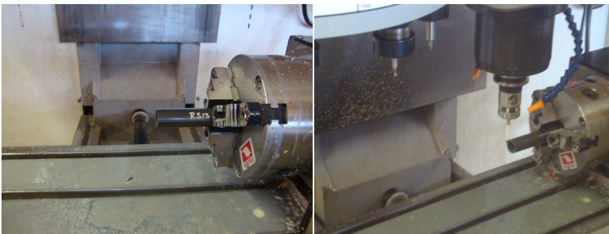
Figure 5-5-9: Photos of a mounted pipe being prepared for profile cutting
