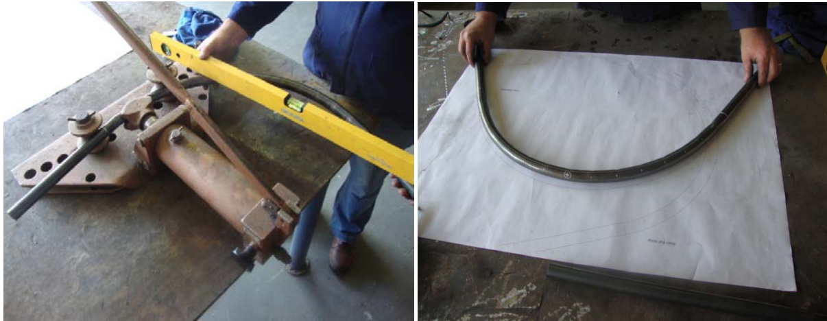
Figure 5-14: Bending of the main and front roll hoops
