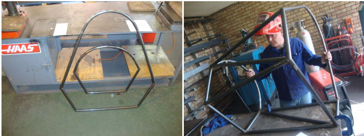
Figure 5-15: Photos of the roll hoops and cockpit structure construction
