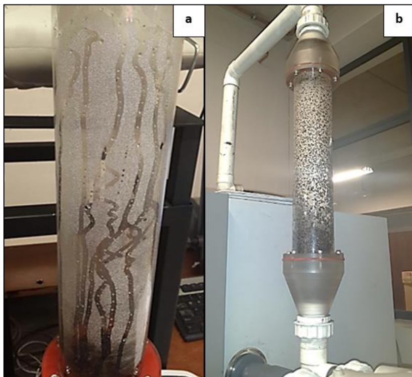
Figure 5.4.2(a) Condensate and (b) fine coal adhering to the side of the fluidized bed
