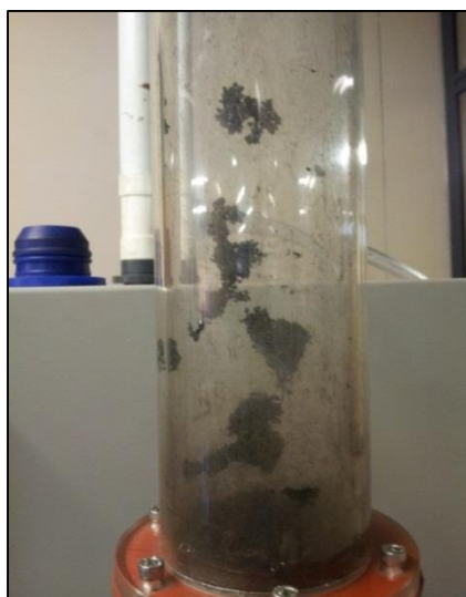
Figure 5.4.1 Agglomerates adhering to the side of the fluidized bed
