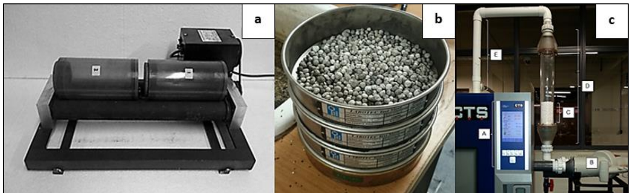
Figure 5.3.2 Photographs of the rotating bed (a), sieves (b) and packed bed (c)
