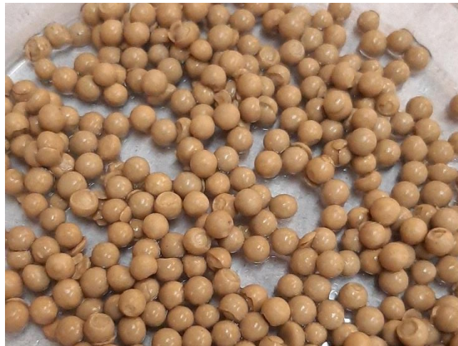
Figure 5-37 Molecular sieves' brittleness and particle breakage
