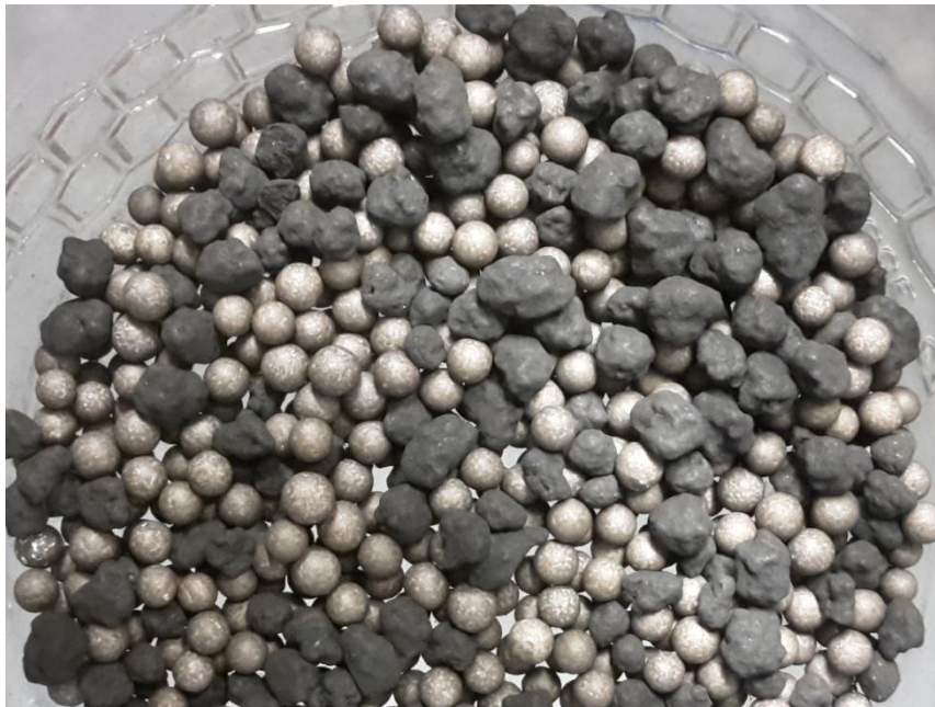
Figure 5-33 Small lumps of flotation product coal with activated alumina
