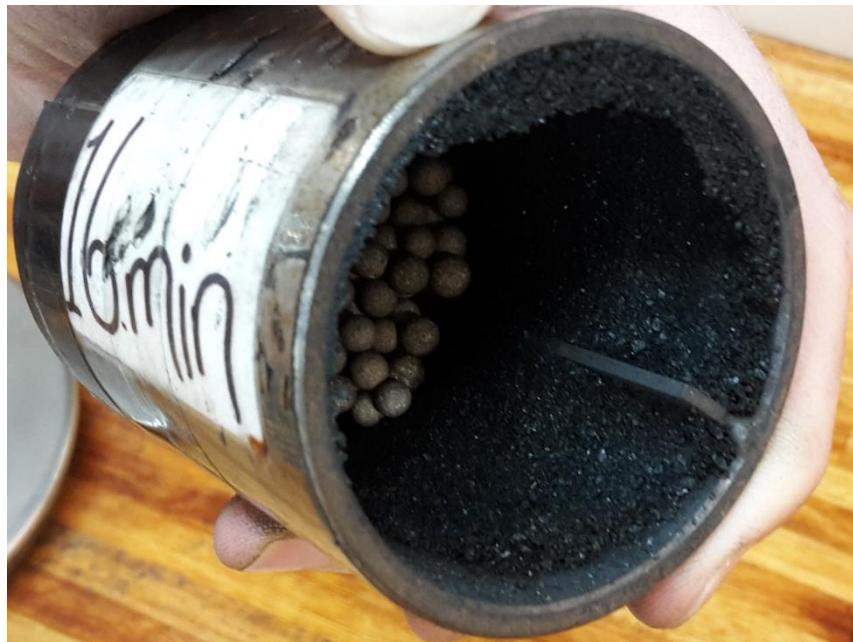
Figure 4-30 Spiral coal caking against a cylindrical vessel's inner wall
