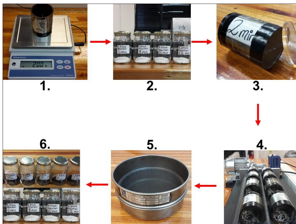
Figure 3-11 Adsorbent assisted drying procedure
