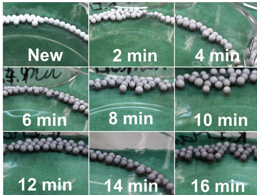
Figure 4-31 Coal dust entrapment on the adsorbents' surfaces as usage progresses
