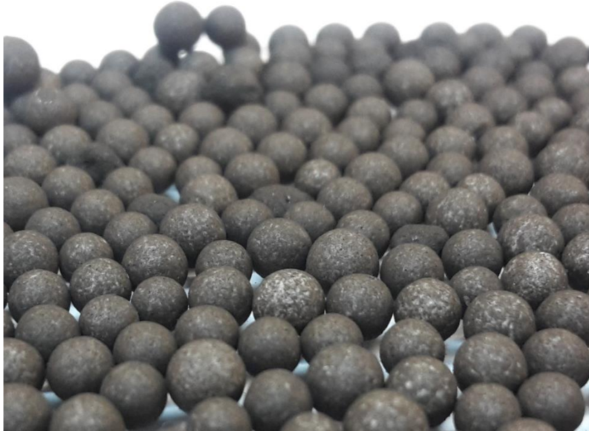
Figure 5-34 Coal dust entrapment on flotation product's spent activated alumina
