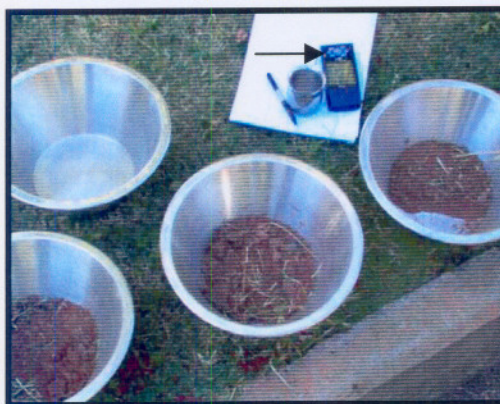
Figure 2.3: Some of the equipment used during sampling in the field. This photo shows the GPS (indicated by an arrow) used to locate the sampling positions and the stainless steel containers used to collect the composite samples.
