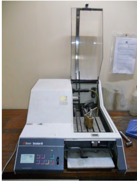
Figure 22: Struers' Secotom-10 used to section the samples
