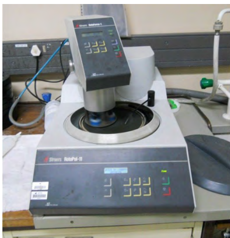
Figure 25: Struers Rotopol-11 machine used for grinding and polishing of samples
