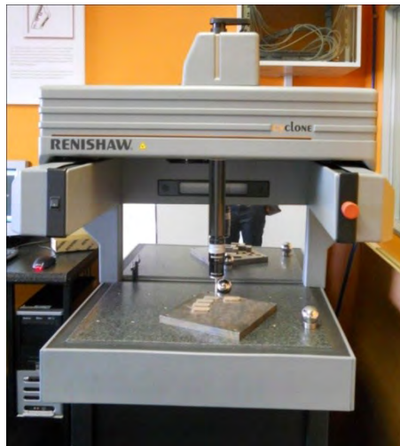
Figure 43: Samples being traced with the Renishaw Cyclone CMM
