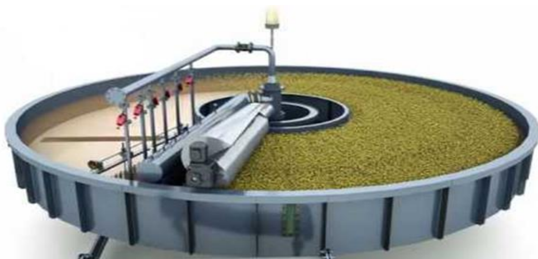
Figure 7: Dissolved air flotation with solid-liquid separation
