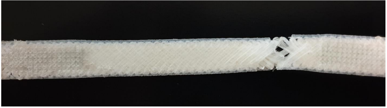
Figure 33: 45°/135° fibre orientation specimen post-testing
