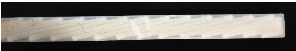
Figure 43: 10^\circ fibre orientation specimen post-testing
