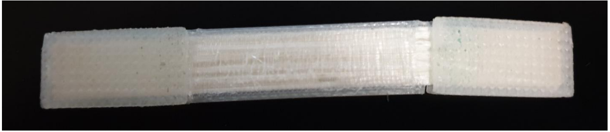
Figure 20: ASTM D3039 Tested specimen with tabs
