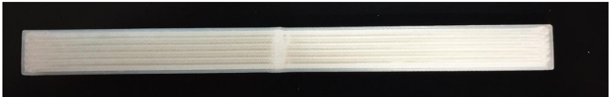
Figure 29: 0° fibre orientation specimen post testing
