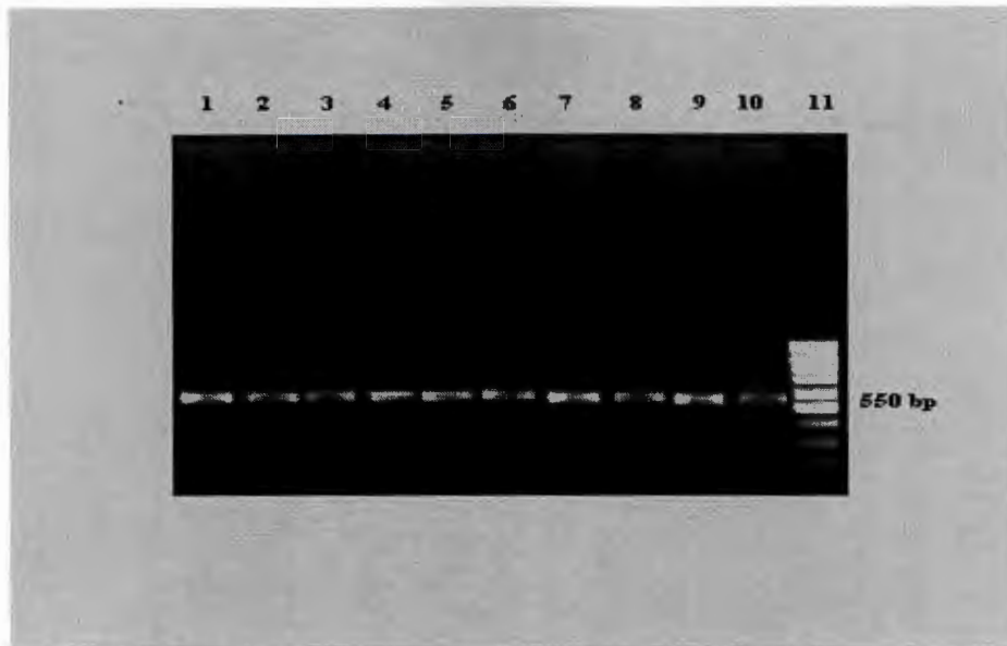
Figure 4.6: Image of an agarose (1% w/v) gel indicating 16S rRNA gene fragments generated by PCR analysis using genomic DNA extracted from E. coli O157 isolated from the various species and E. coli control strains. Lanes 1-3 (16S rRNA gene fragment from DNA extracted from E. coli O157 isolated from cattle –Rustenburg, Lichtenburg and Mogosane respectively); Lanes 4-5 (16S rRNA gene from DNA extracted from E. coli O157 isolated from pigs – Mareetsane); Lanes 6-7 (16S rRNA gene from DNA extracted from E. coli O157 isolated from pigs – Tlapeng); Lane 8 (16S rRNA gene fragment from DNA extracted from E. coli isolated from human stool samples – Mafikeng Provincial Hospital); Lanes 9-10 (16S rRNA gene fragment from DNA extracted from E. coli O157:H7 (ATCC 43889) and E. coli O157:H7 (ATCC 43888) control strains respectively. Lane 11 (100 bp –DNA Ladder).
