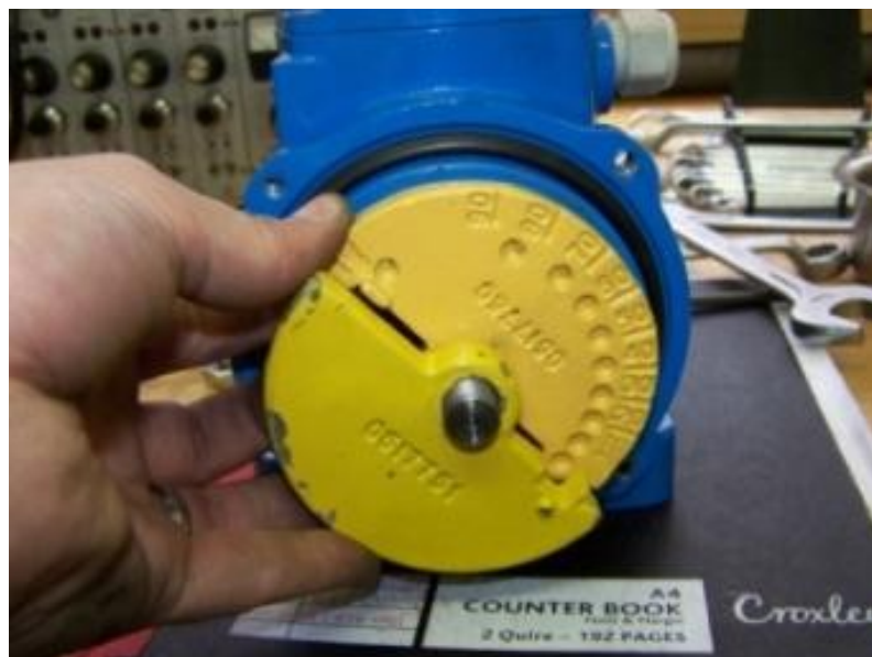
Figure 39: The adjustable unbalance plates on the vibrating motor
