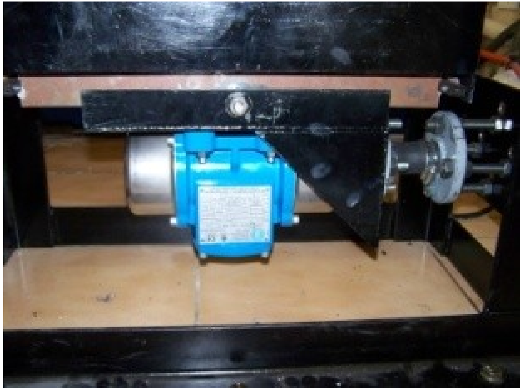
Figure 38: The electric vibrating motor, used to induce the forced frequency
