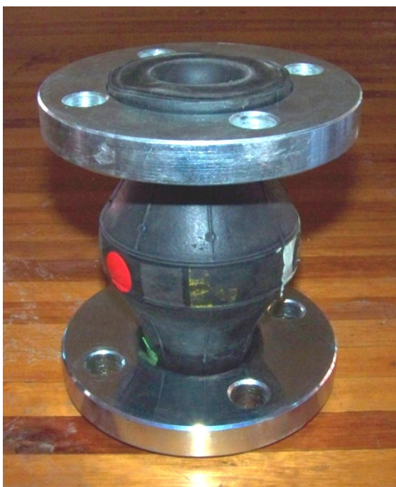
Figure 47: An image of the selected pipe compensators used in the experiment
