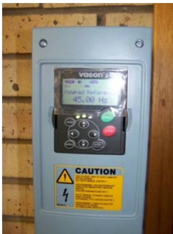
Figure 40: The speed control used to control the forced frequency of the model
