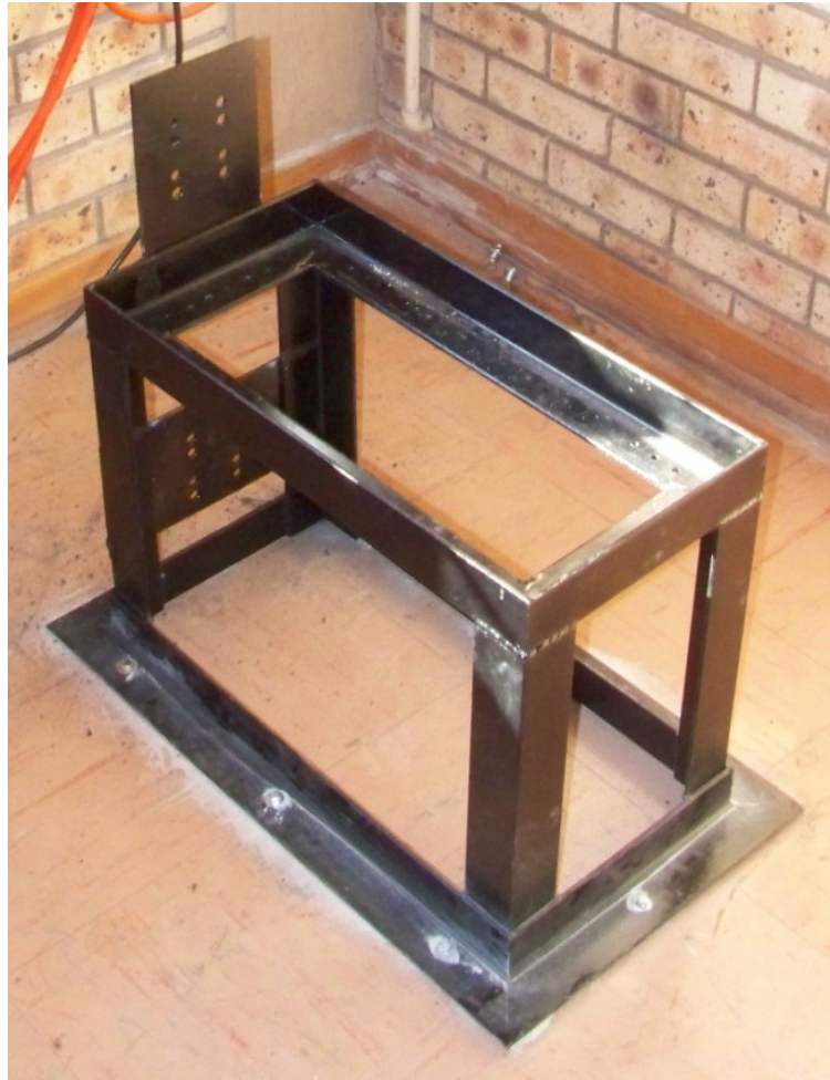
Figure 45: Support frame Rawl-bolted to the floor
