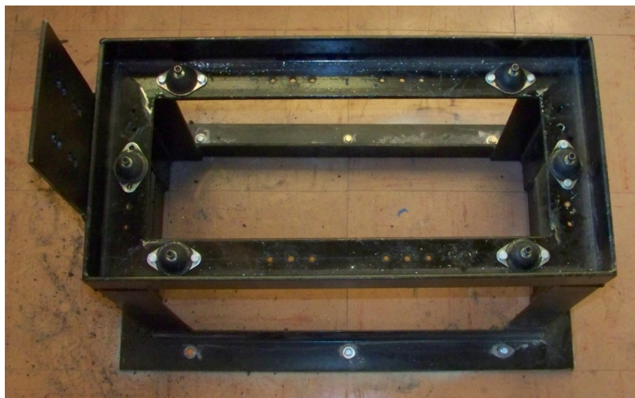
Figure 46: Soft rubber mounts used to isolate the heat exchanger from the support structure
