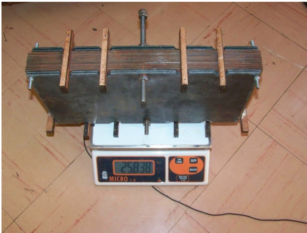
Figure 42: The assembled plate pack with Masonite guides
