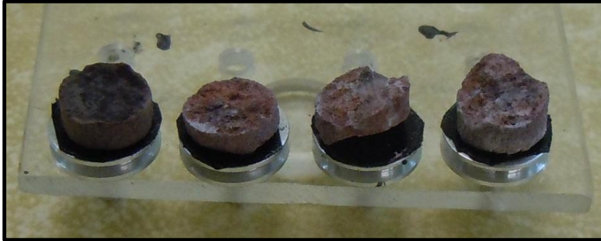
Figure 75 - Catalyst Pellets Cut through the Midsection to Analyse their Cross-section and Poison Penetration Depth
