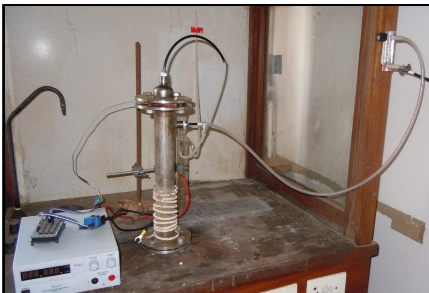
Figure 93 - Activation Oven Setup
