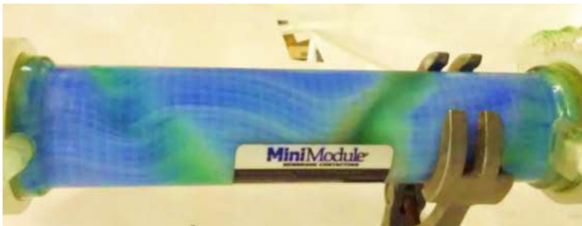
Figure 4-4: A colour-enhanced photo illustrating shell-side channelling (large green bands) and lumen-side maldistribution (vertical striations in blue fibres). Note that the photo has been rotated 90° counter-clockwise for the purposes of this document, under normal conditions the module was oriented upright with the bottom shell-side inlet seen on the right of the clamp.
