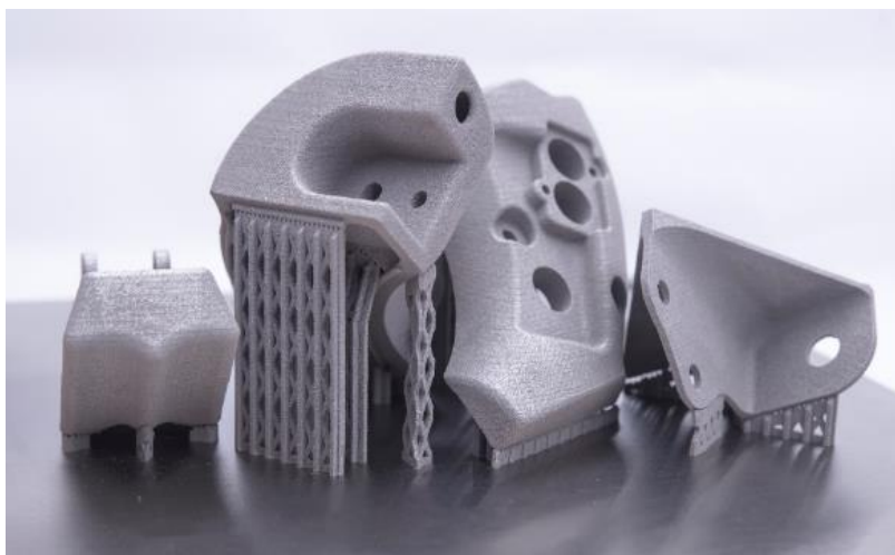
Figure 2-8: Parts built on the Aeroswift machine
