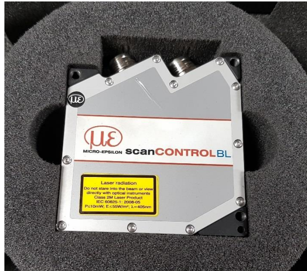
Figure 3-5: Micro-Epsilon's ScanCONTROL 2960-50/BL
