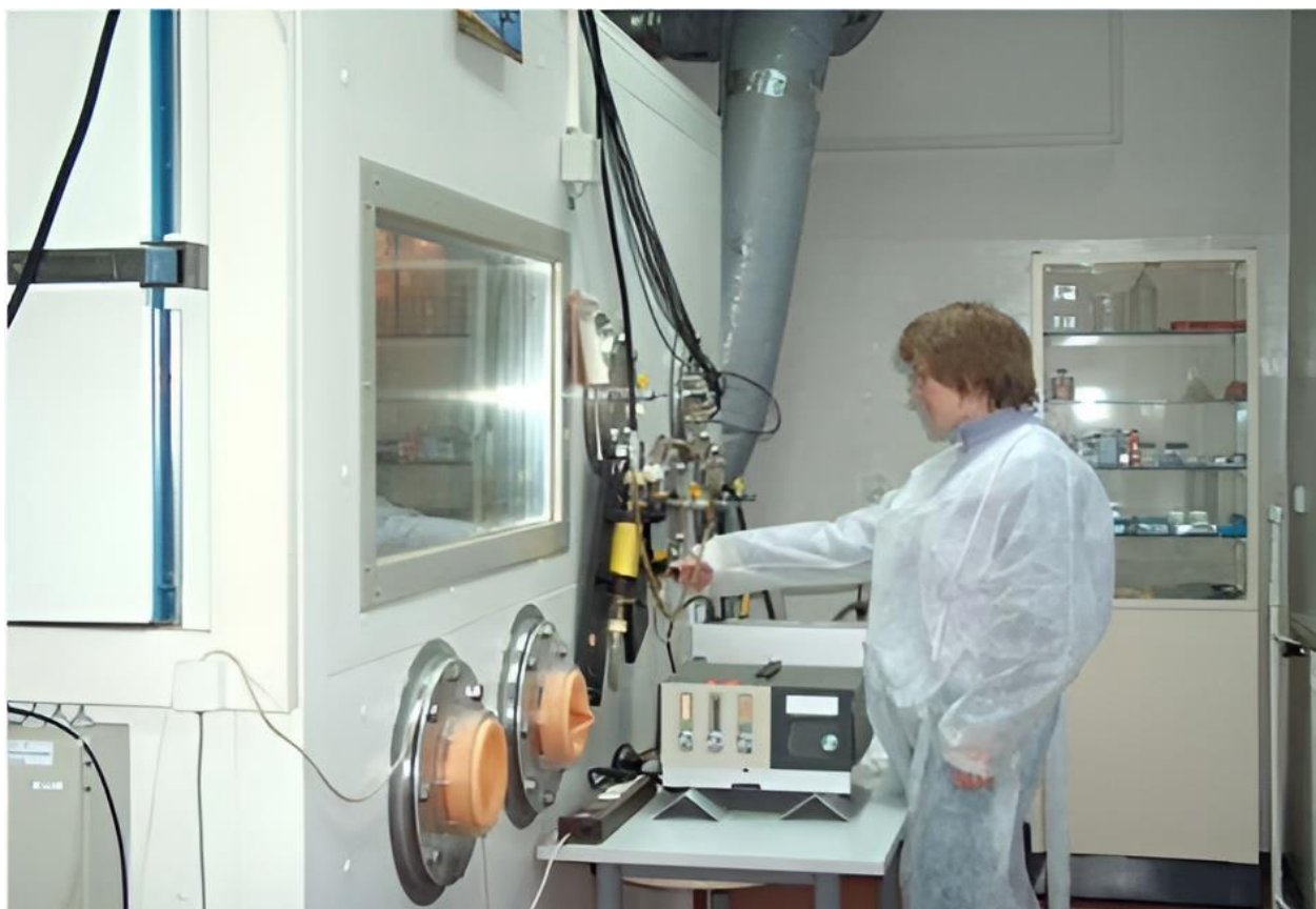
Figure 2.13: Walk-in radon chamber (Mamont-Cieřla et al., 2010).
