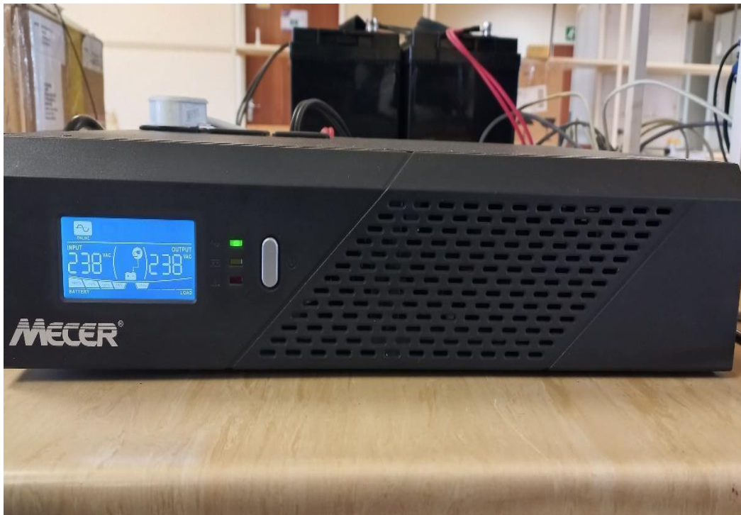
Figure 3.6: Mecer 2400va inverter for uninterrupted experimental measurements during load shedding.
