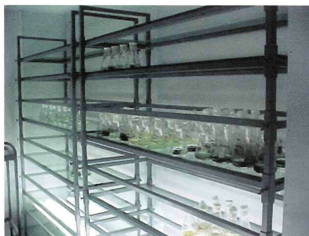
Figure 4.6: Cultures grown in 100 ml of culture medium in regulated chambers at a constant temperature (18°C) and light (20 μmol.m -2 .s -1 ).
