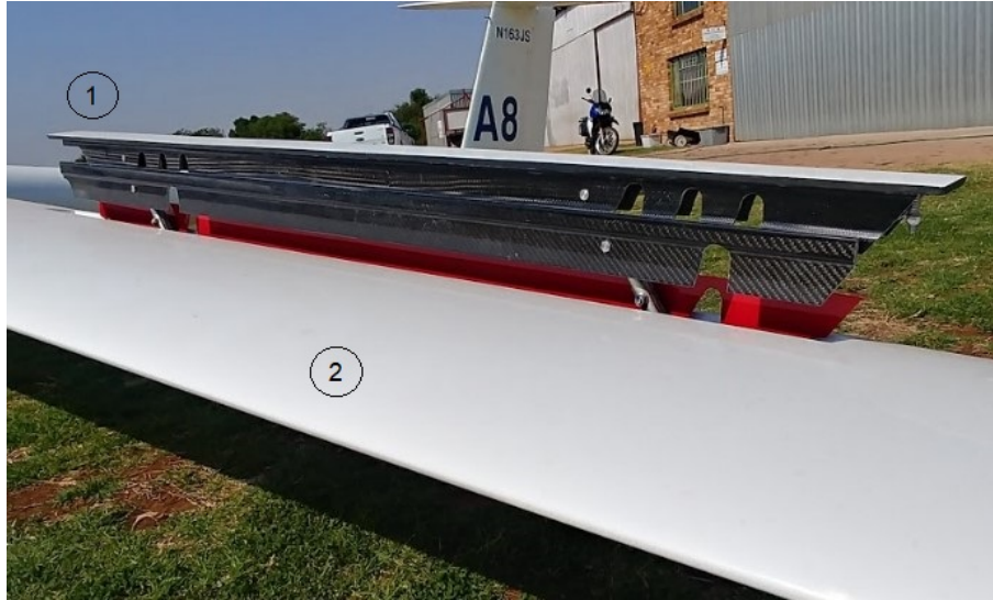
Figure 1.2: Schempp-Hirth type airbrakes used on the JS3 sailplane.
