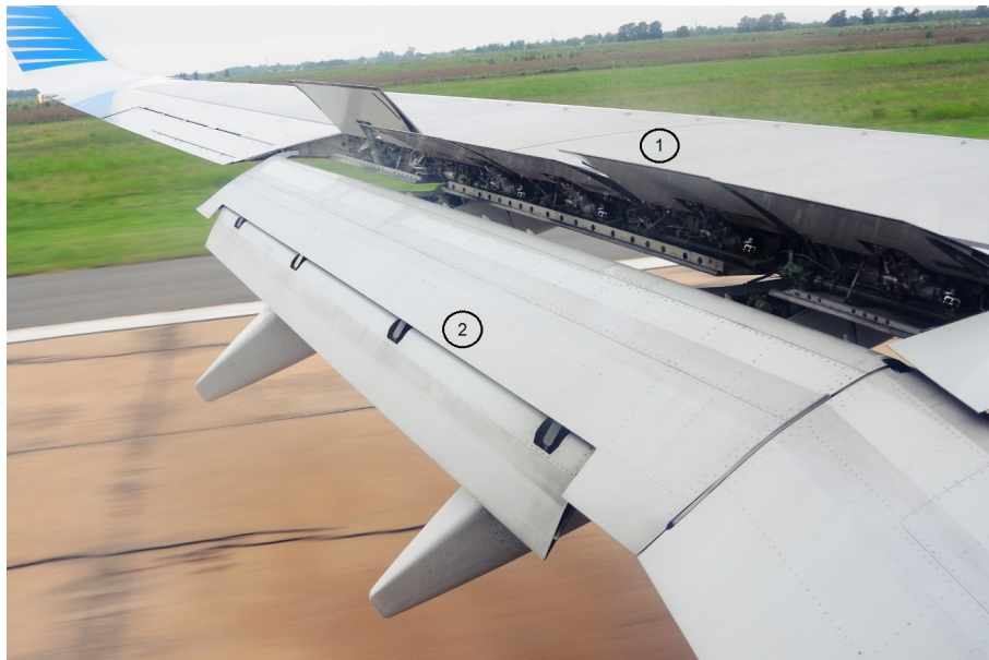
Figure 1.1: Spoilers and Flaps extended of a Boeing 737-700 [1]
