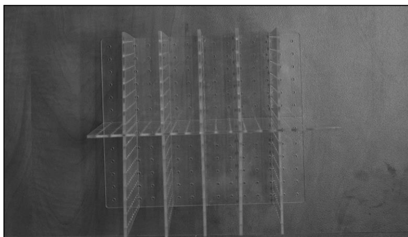
Figure 3-2 - Schematic (above) and photographic (below) view of home cage setup and separators, respectively, allowing for simultaneous fish identification and social interaction.
