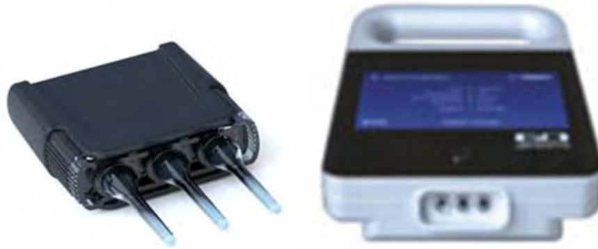
Figure 2: Components of the Genedrive system developed by Epistem. Test cartridge (left) and Genedrive instrument (right). Images (advertorial) reprinted from Epistem (UK). https://www.genedrive.com/ . Date of access: 6 January 2016
