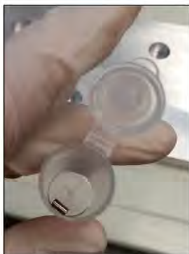
Figure 2: The lysis micro reactor (LMR)
