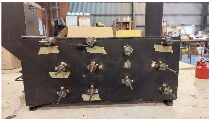
Figure A-2: Thermocouple fittings were placed on the Flamingo™ stove.
