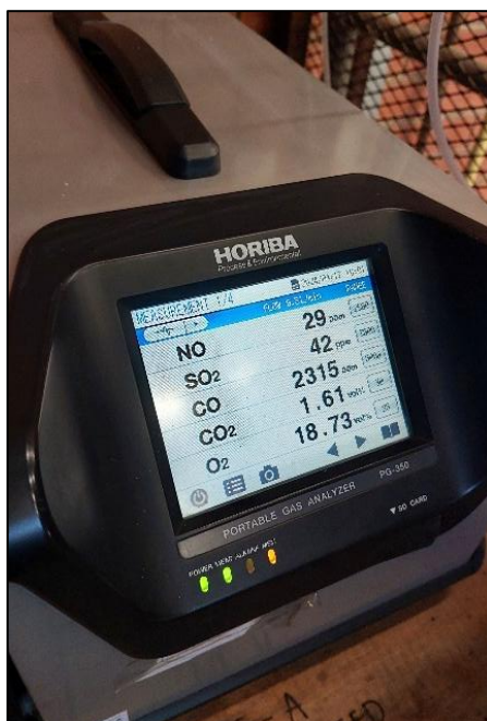
Figure 3-9: Horiba PG350 gas analyser display.
