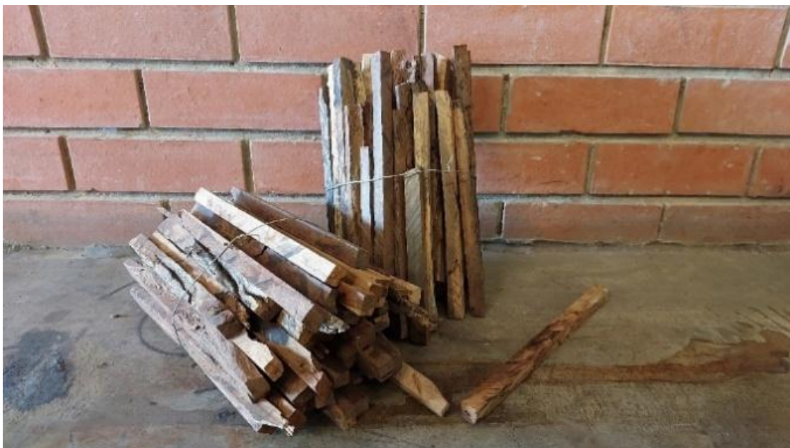
Figure 3-1: Mopane wood cuttings used in the Flamingo™ stove tests.
