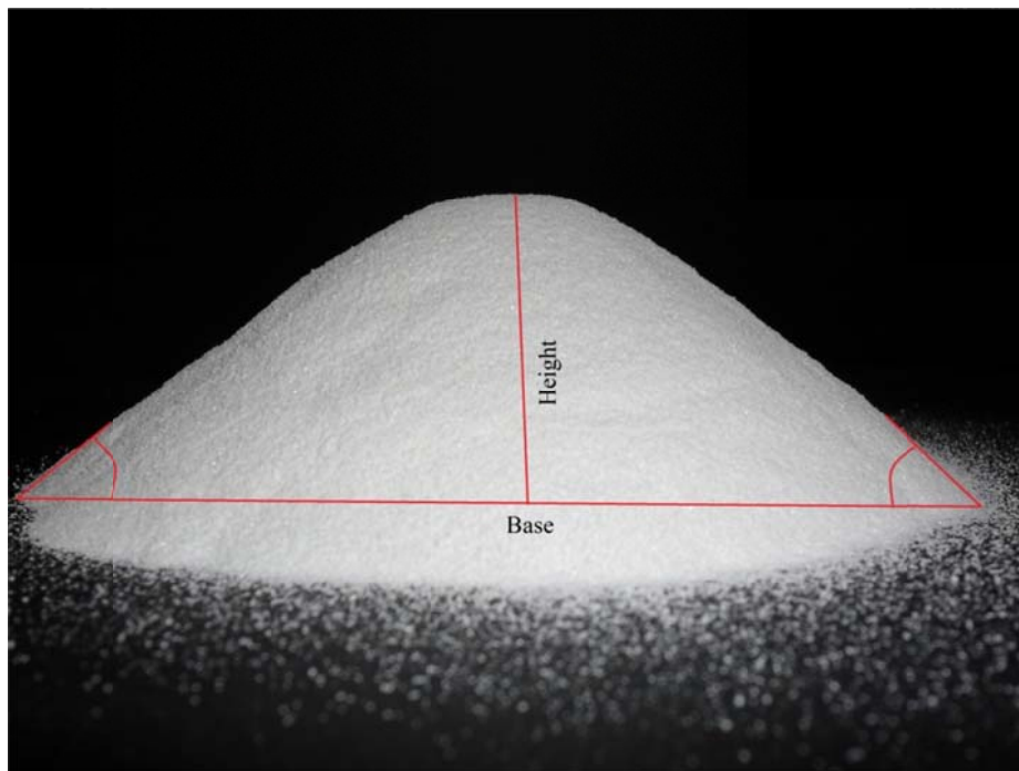
Figure 4.3: Powder conical heap with reference lines to enable measurement of its height and base for the angle of repose calculation.
