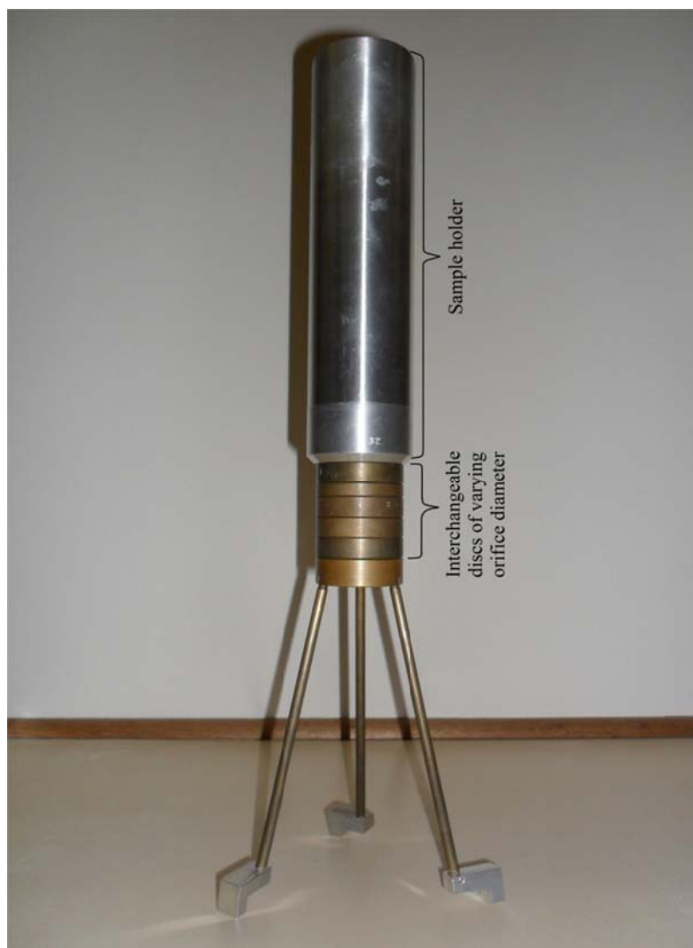
Figure 4.4: The apparatus developed by Buys (2006) for use in the determination of the critical orifice diameter.
