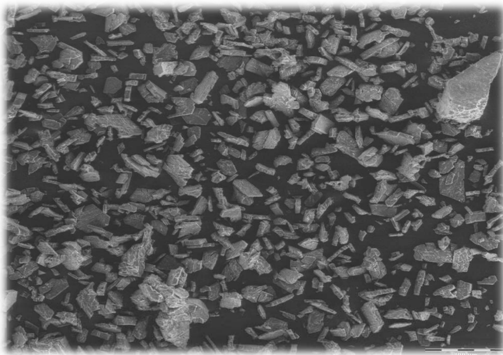
Figure 1.5: SEM Photomicrographs of nevirapine powder subjected to novel method of size reduction
