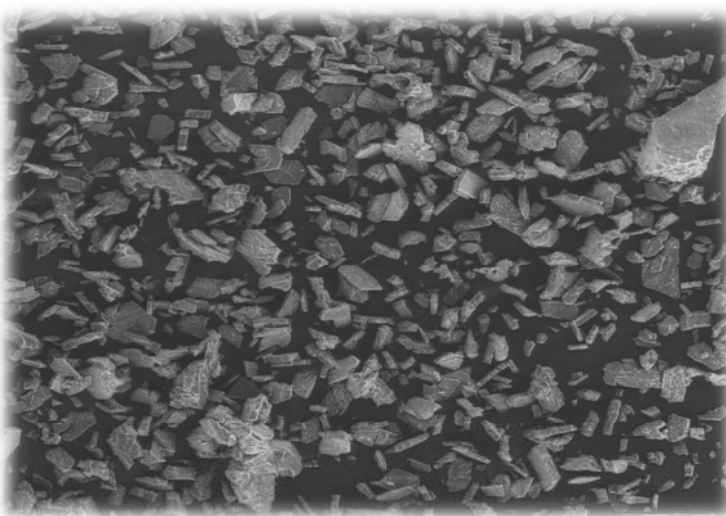
Figure 5.2: SEM photomicrograph of fine nevirapine powder (novel method of preparation).
