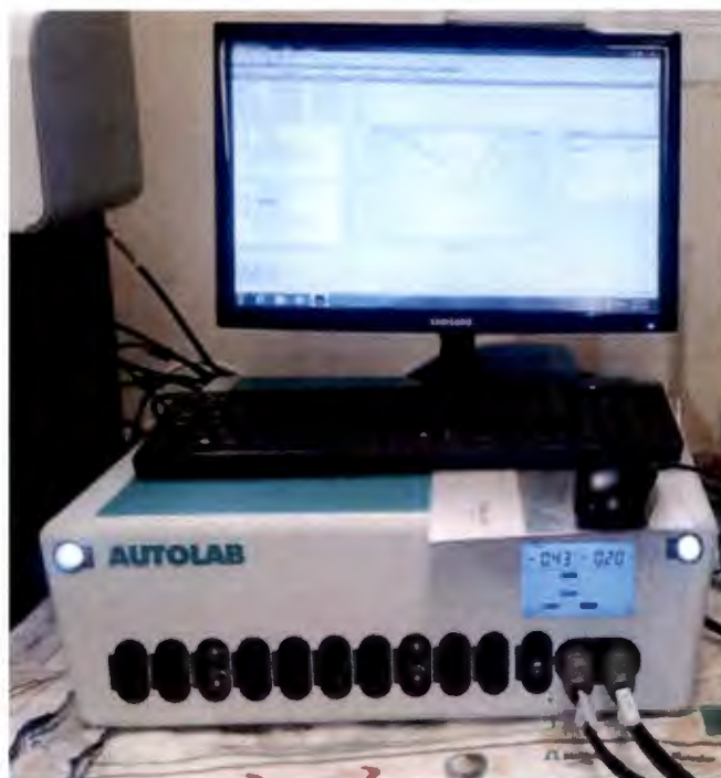
Figure 3.2: Autolab setup for electrochemical measurement
