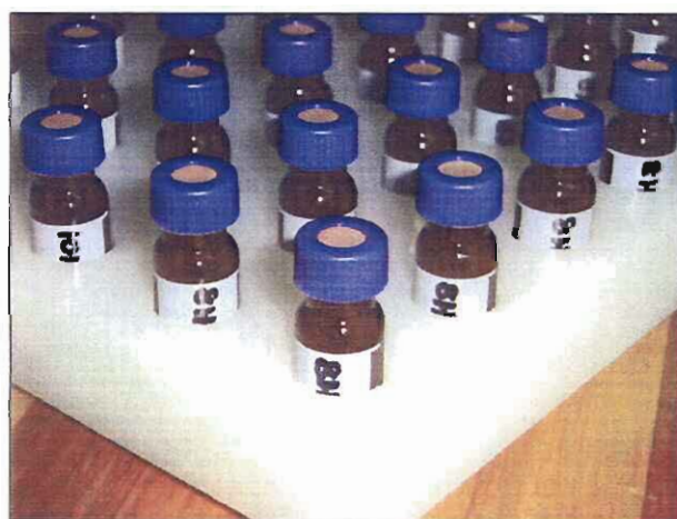
Photo 7: Separations® amber HPLC vials used to collect samples
