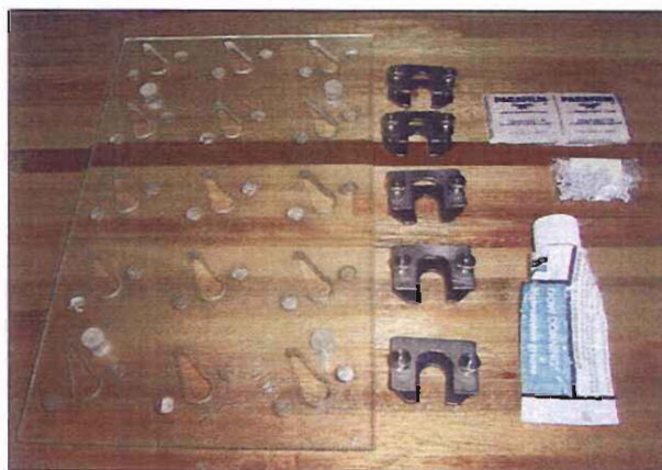
Photo 2: Franz cell stand, metal clamps, parafilm®, magnetic stirrer bars & Dow Corning® vacuum grease
