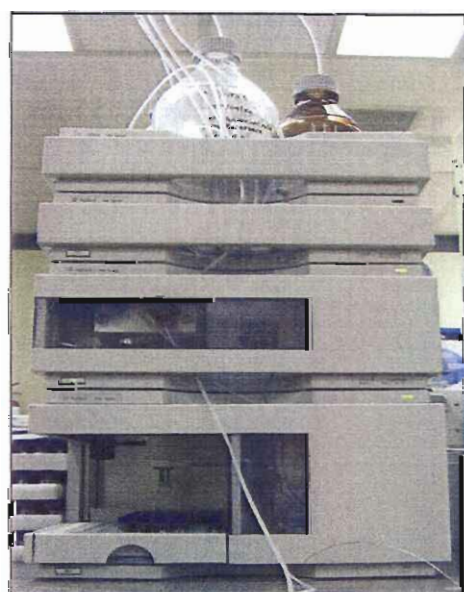
Photo 9: Agilent® series 1100 HPLC
