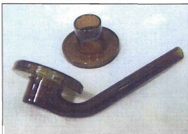
Photo 1: Amber Franz cell (donor & receptor compartments)
