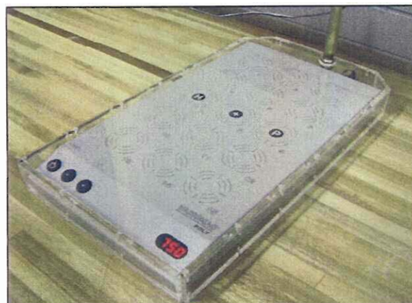
Photo 6: Variomag® magnetic stirrer plate
