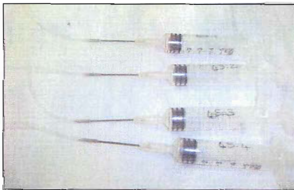
Photo 4: Syringes used to withdraw the receptor compartment fluid
