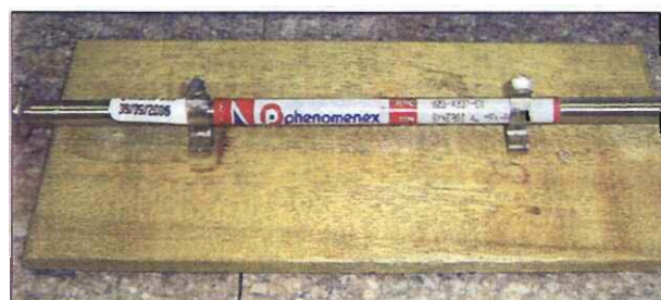
Photo 8: Phenomenex®, Synergi Max RP-80A, 250 x 4.6 mm, 4 µm column
