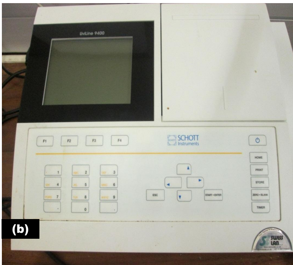
Figure 3.3. The UV-Vis spectrophotometers (a) Cary UV-Vis, and (b) UViLine 9400 used for the UV-Vis studies.
