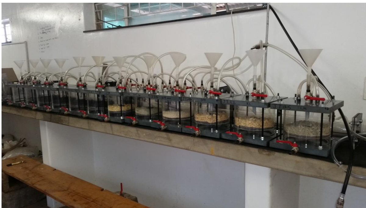
Figure 3.6: Humidity cell leaching experiment set up, showing moist air outlets, water heater and air supply. Photograph taken by Mphinyane (2017), Spoor Lab, North-West University.
