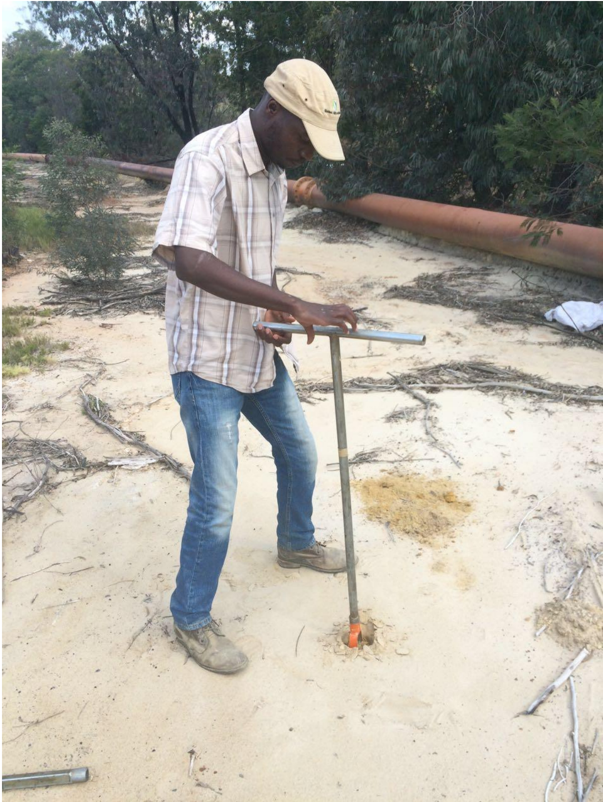
Figure 3.4: Sampling at the bench of a slope of the tailings dam, Crown mine, South Africa. Photograph taken by Kruger (2016), with permission.
