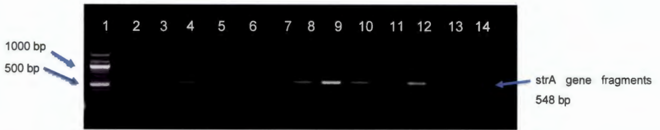
Figure 4.4: An image depicting a 1.3% (w/v) agarose gel of the strA gene fragments amplified from isolates. Lane M= 100 base pairs DNA ladder; Lanes 1-11 and 13-14: strA gene fragments of representative isolates and Lane 12: No template DNA negative control reaction.
