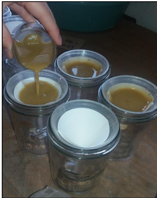
Figure 21: Photograph illustrating the preparation of the filtrate used to measure \text{pH}(\text{H}_2\text{O}) .
