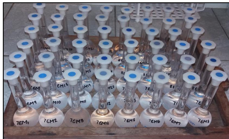
Figure 24: Volumetric flasks containing 5 ml Bray-1 extract and 45 ml Lanthanum solution.
