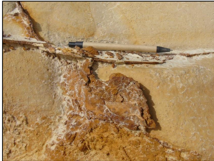
Figure 7: A photograph of ferrihydrate (rusty brown iron hydroxide mineral) on the surface of a gold TSF. Photograph taken by Schimmer (2016), with permission.
