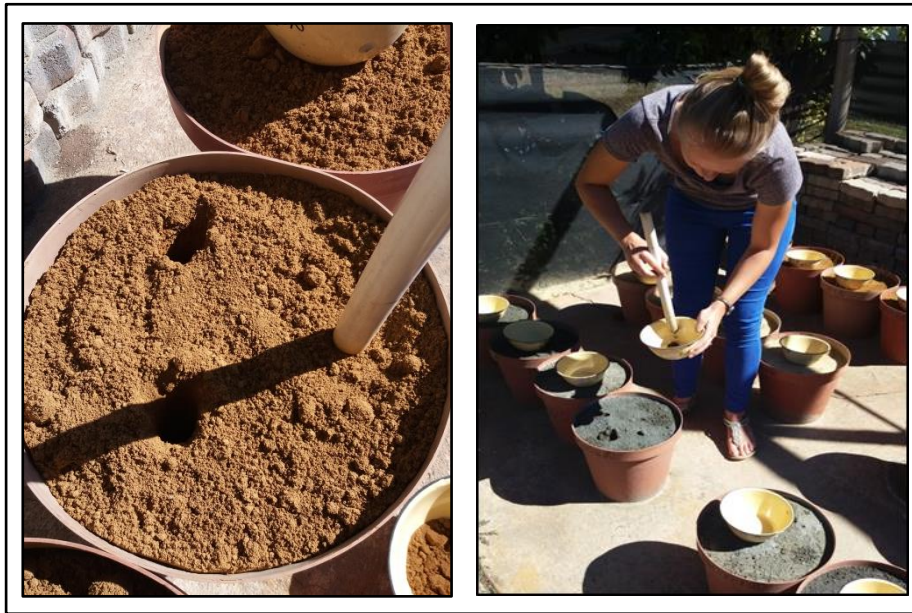
Figure 18: Photographs showing the process of composite sampling of the material with the use of a PVC pipe. Photographs were taken by De Necker (2017), with permission.
