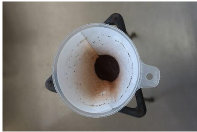
Figure 2.14 Sample drained into the wash trough with the ring of cysts and debris formed on the inner sides of the filter paper funnel (Photo by S. P. Swart).
