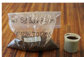
Figure 2.4 Sample bag with soil and roots, together with a beaker with 250g soil. This is ready for the start of the sieving centrifugal flotation method (Photo by S.P. Swart).
