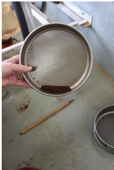
Figure 2.11 Debris and cysts collected on a 150 \mu\text{m} aperture sieve (Photo by S. P. Swart).
