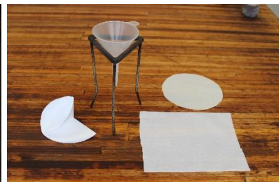
Figure 2.19 The funnel in preparation, the Whatman filter paper already folded in quarters to be put into the funnel (Photo by S.P. Swart).
