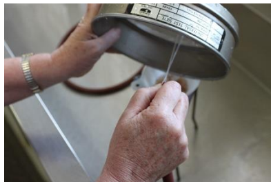
Figure 2.12 Debris and cysts were transferred from the 150 \mu\text{m} aperture sieve to the filter paper that fitted snugly in the plastic funnel into the funnel (Photo by S.P. Swart).
