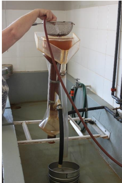
Figure 2.9 The soil sample containing cysts being washed through the 2-mm aperture sieve (Photo by S.P. Swart).
