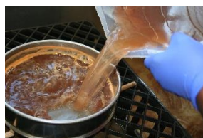
Figure 2.5 Soil sample washed through a 45 µm sieve during the sieving centrifugal flotation method (Photo by M. Marais).
