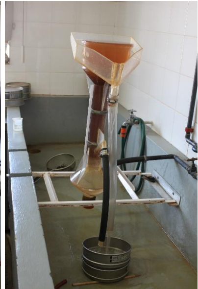
Figure 2.10 The water (and debris) spills over the collar through the upper downpipe aperture sieve (Photo by S.P. Swart).
