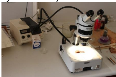
Figure 2.17 The filter paper on the plastic plate is put on the stage of a dissection microscope to be viewed (Photo by S. P. Swart).
