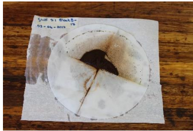
Figure 2.15 The filter paper funnel opened into a circle and dried on a paper towel (Photo by S. P. Swart).
