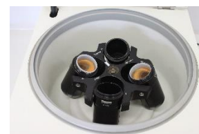
Figure 2.7 Centrifuge tubes are filled with the extracted soil sample, ready to be centrifuged for 7 minutes at 3500 revolutions per minute (Photo by S.P. Swart).
