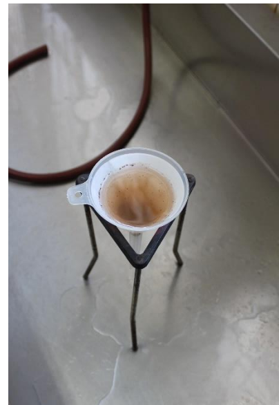
Figure 2.13 Sample in the funnel, draining into the wash trough (Photo by S.P. Swart).
