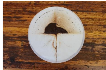
Figure 2.16 The filter paper, still damp, put on a round, plastic plate (Photo by S.P. Swart).
