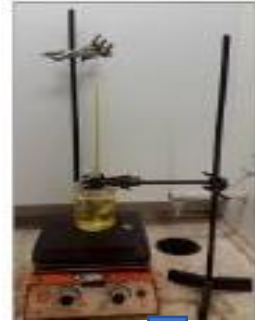
Methanolysis Temperature 27 °C – 60 °C Residence time 6 – 24 hours
