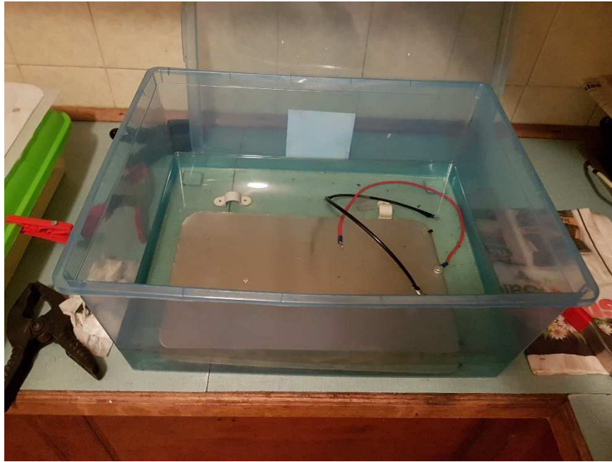
Figure 5-13: Charged plate submerged in transformer oil.
