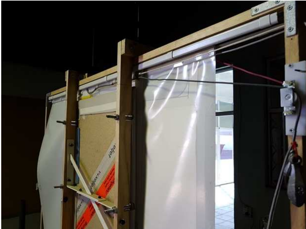
Figure 5-11: Stuck electrode due to electrostatic forces.
