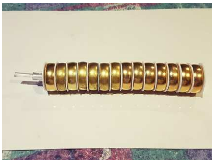
Figure 4-30: Attempt at a segmented Faraday cage cable.
