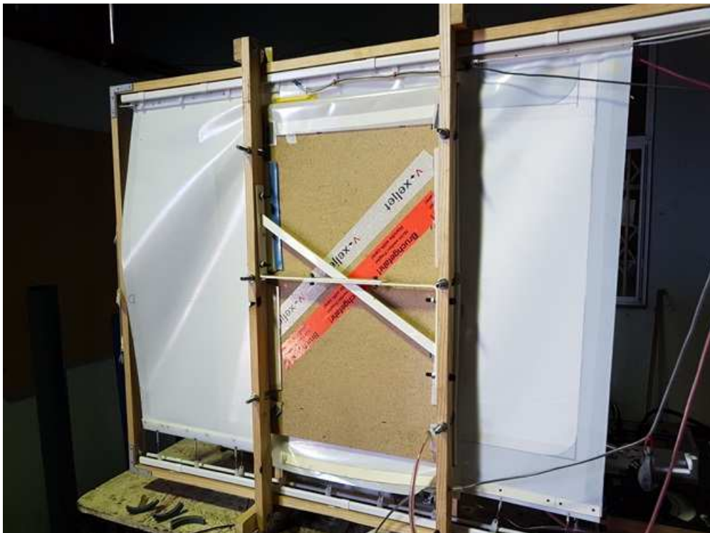
Figure 5-12: Stuck electrode due to electrostatic forces.
