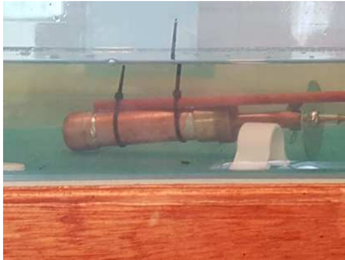
Figure 4-26: Cabling into hollow electrode.
