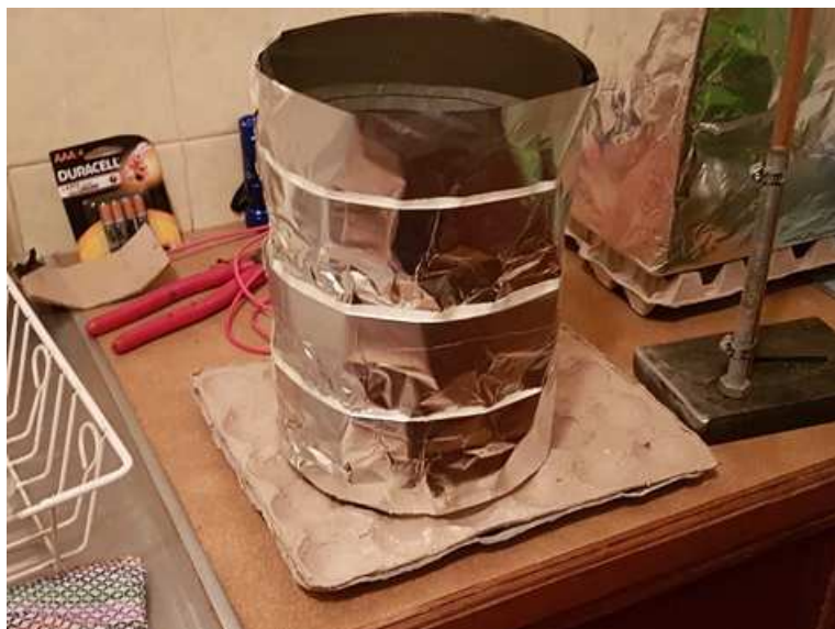
Figure 4-27: First attempt at a segmented Faraday cage.
