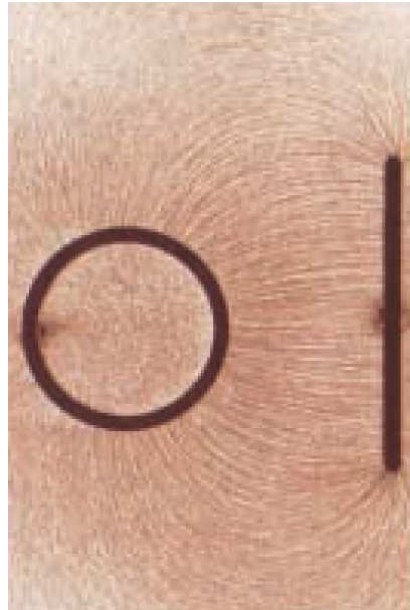
Figure 2-69: Electric field visualisation between cylinder and plate (Tipler & Mosca, 2004: 705).
