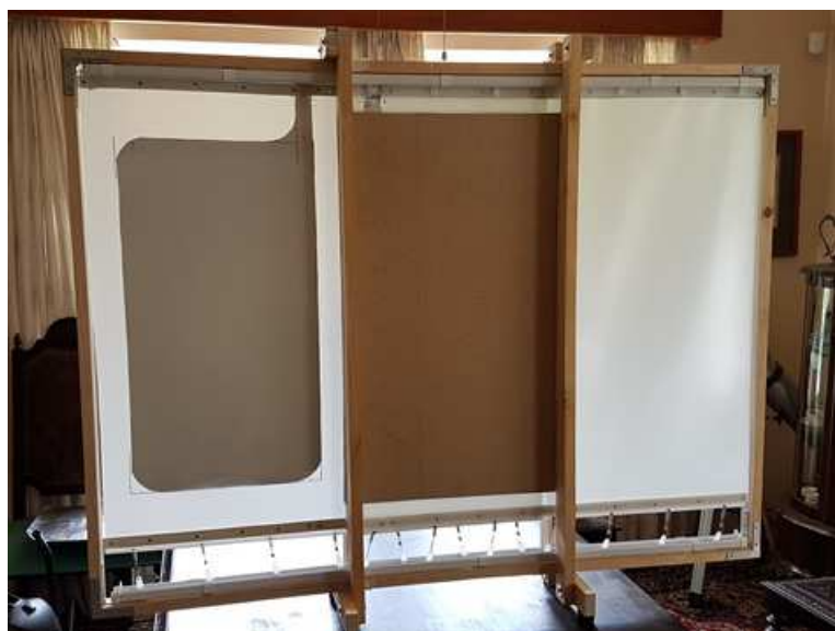
Figure 4-19: Sliding electrode apparatus during construction.
