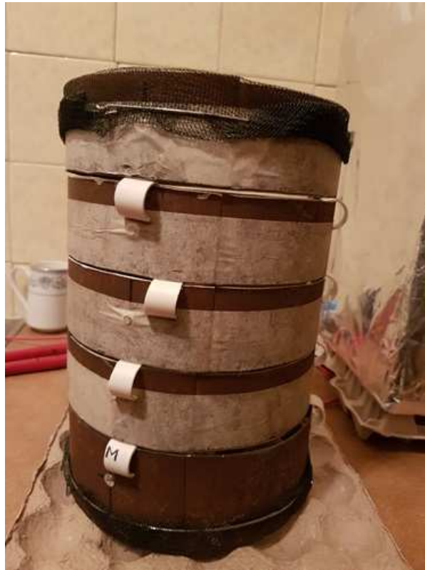
Figure 4-28: Second attempt at a segmented Faraday cage.
