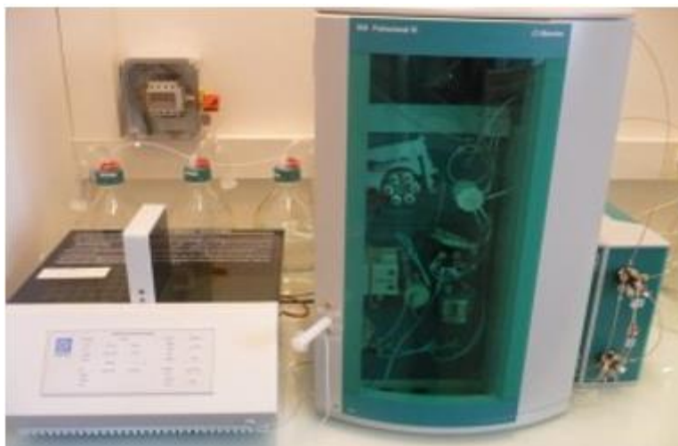
Figure 2-8. The Metrohm IC 850 device (injection loop of 100 \mu\text{l} ) used for ion chromatography analyses at LISA. Photo by: Fadi Lahmidi.
