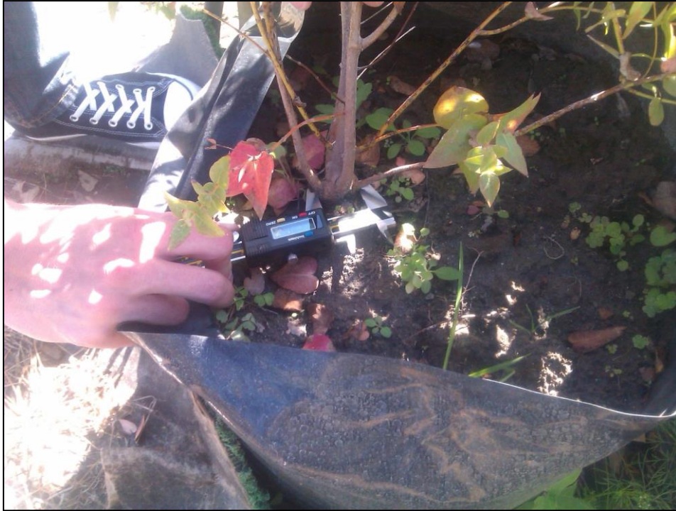
Figure 16: Measurement of basal diameter using an electronic caliper
