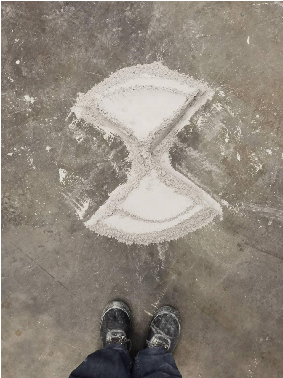
Figure M8: An example of the sample during coning and quartering
