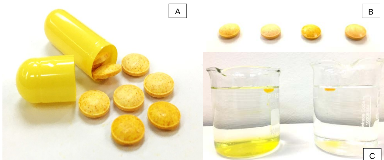
Figure 4-14: (A) A representation of the final mini-tablet in capsule system formulated for this study (B) From left, curcumin-HP \beta CD complex and curcumin immediate release mini-tablets and curcumin- HP \beta CD complex and curcumin gastro-retentive mini-tablets (C) Complex (left) and curcumin (right) gastro-retentive mini-tablets floating in acidic buffer (pH 1.2) during the buoyancy test.
