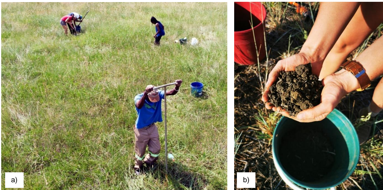
Figure 3.4: a) Soil sampling with the use of soil augers at a sampling site in Vrede (Photo: Dr. Gerhard du Preez, NWU). b) A handful of homogenized soil from ten sub-samples taken at a sampling site in Vrede (Photo: Kelebogile Motlhamme, NWU).
