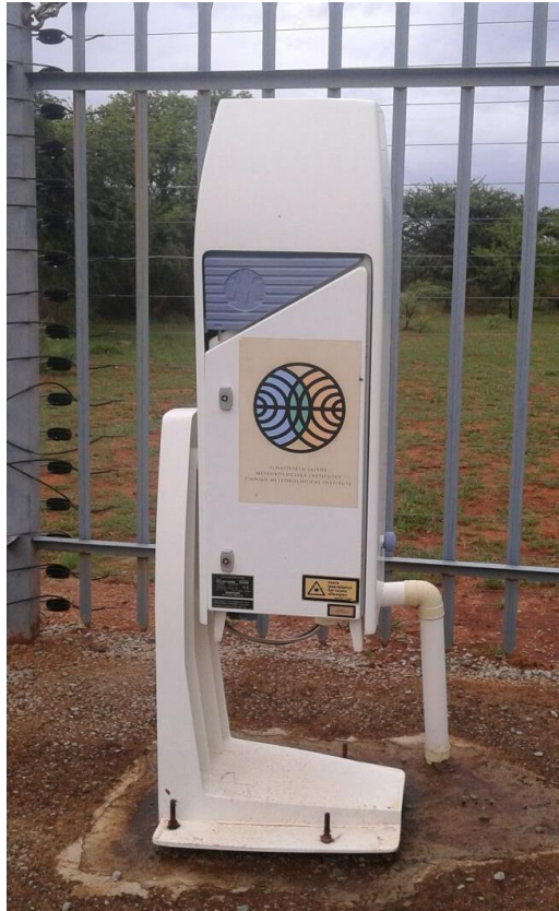
Figure 3.6: The Vaisala CT25K ceilometer (Photo credit: Micky Josipovic)
