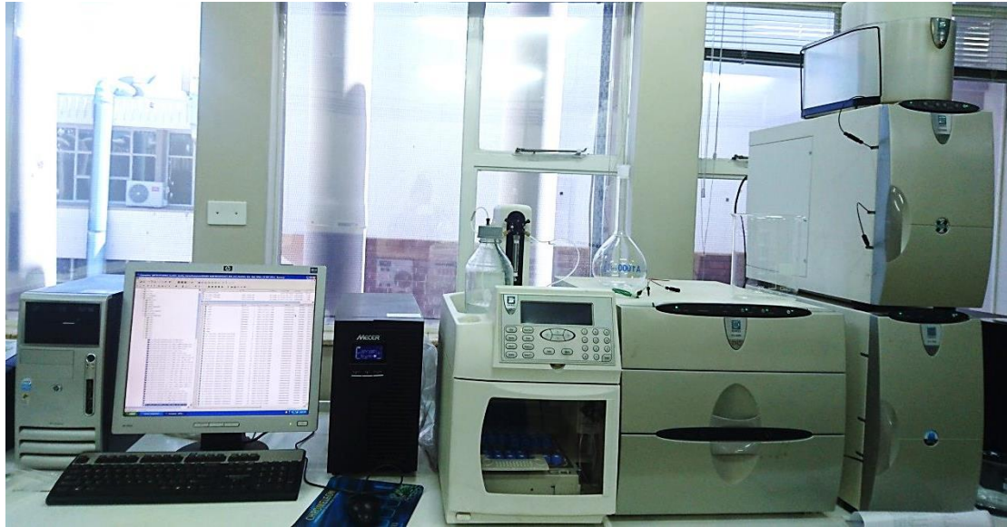
Figure 3.4.1: The Dionex ICS-3000 ion chromatographic system utilised for the ionic content analysis
