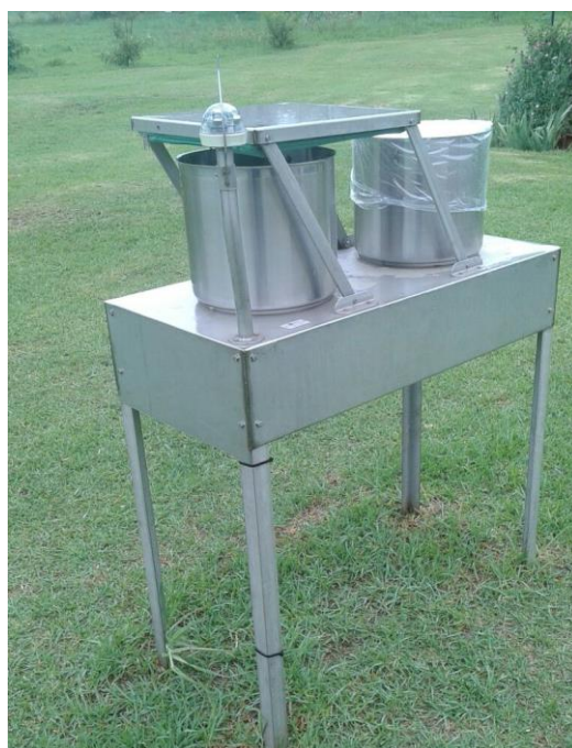
Figure 3.3: The wet-only sampler ( NWU Instrument Makers ). The light-refracting sensor is visible at the foremost corner of the instrument. The instrument is in the “open” position (Photo credit: Micky Josipovic)
