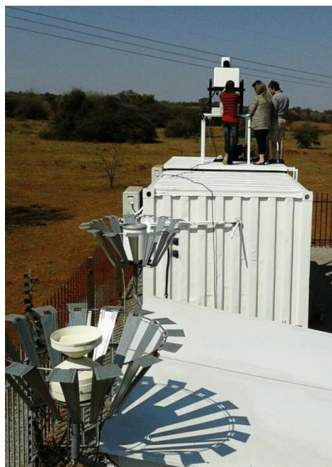
Figure 3.5: The Vaisala QMR102 and Casella 0.1 mm tipping bucket rain intensity instruments as installed at the Welgegund measurement station (Photo credit: Micky Josipovic)
