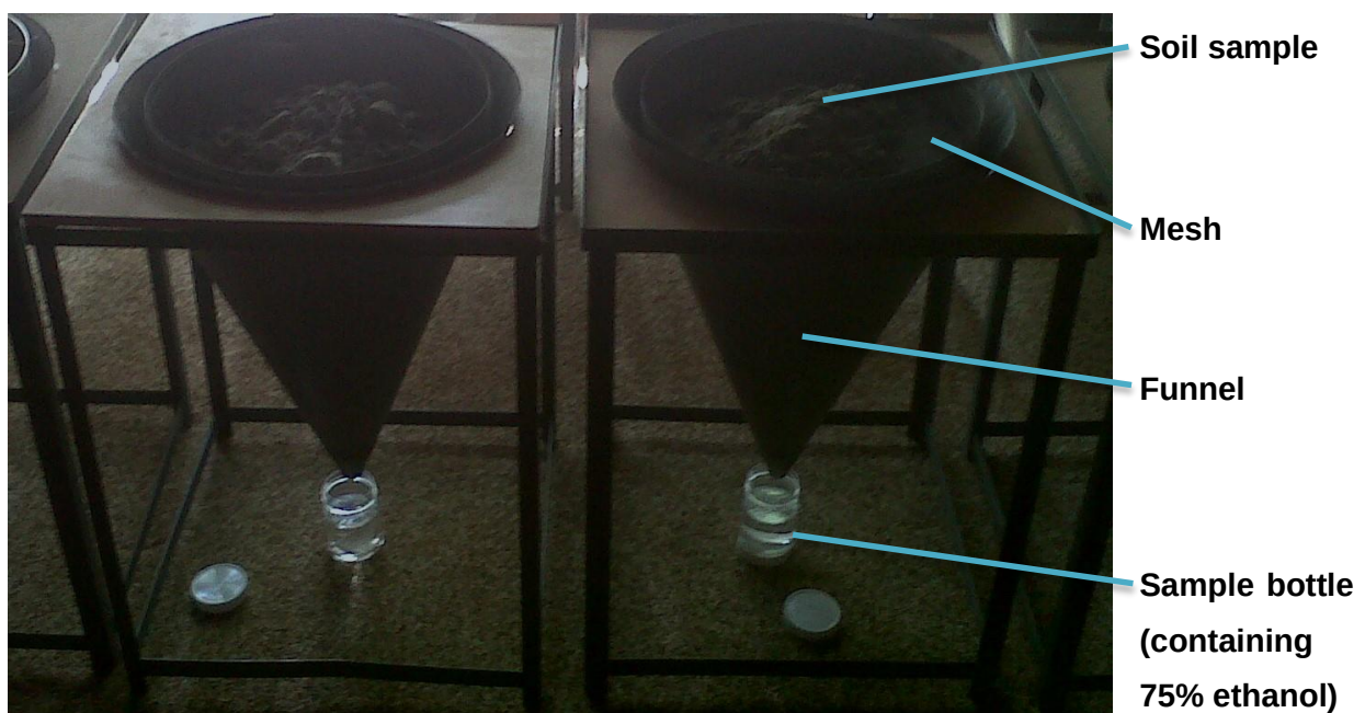
Figure 3-11: Berlese-Tullgren funnels used for extracting terrestrial mesofauna.
