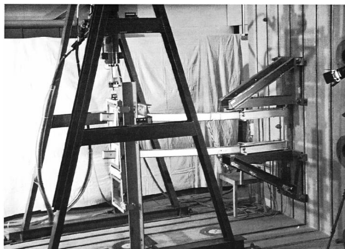
Figure 21: Sailplane Wing Spar Fatigue Test (Kensche, 2002(b))
