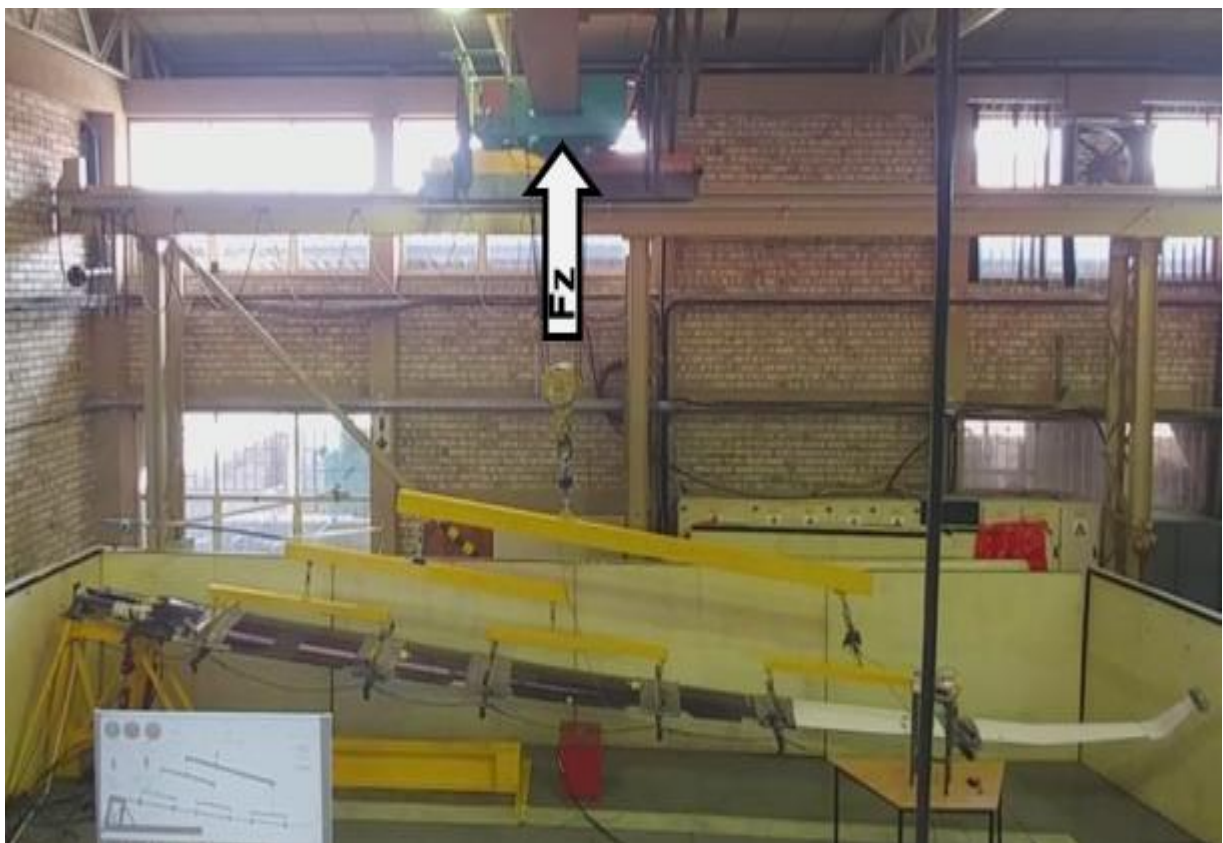
Figure 15: Static Wing Test Setup Example
