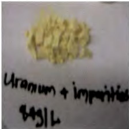
Figure 6.13: Dried precipitate obtained with initial uranium solution concentration of 84 g/l
