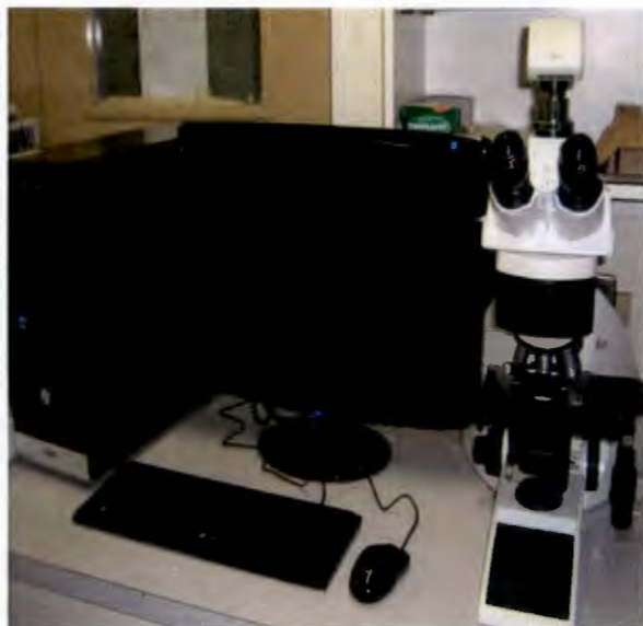
Figure 6.5: Leica DM 4000B for analyzing particles formed.
