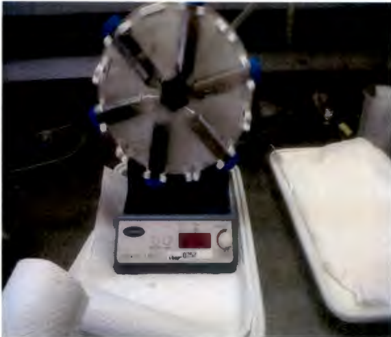
Figure 4.5: Sample rotator with resins shaken for 24 hours
