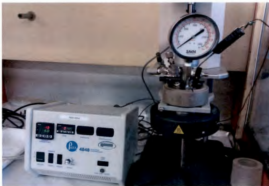
Figure 3.2: Pressurized autoclave that was used to investigate dissolution of UOC
