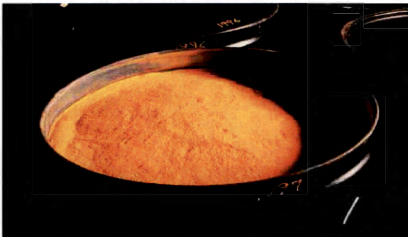
Figure 2.5: The final product of uranium recovery process called yellow cake.
