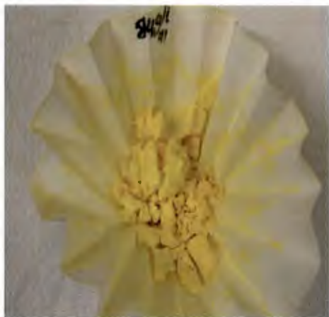
Figure 6.7: Yellow precipitate of uranyl ion
