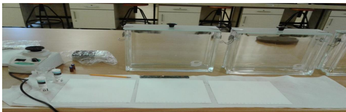
Figure 3.3: Image of standards and samples preparation on silica gel plates
