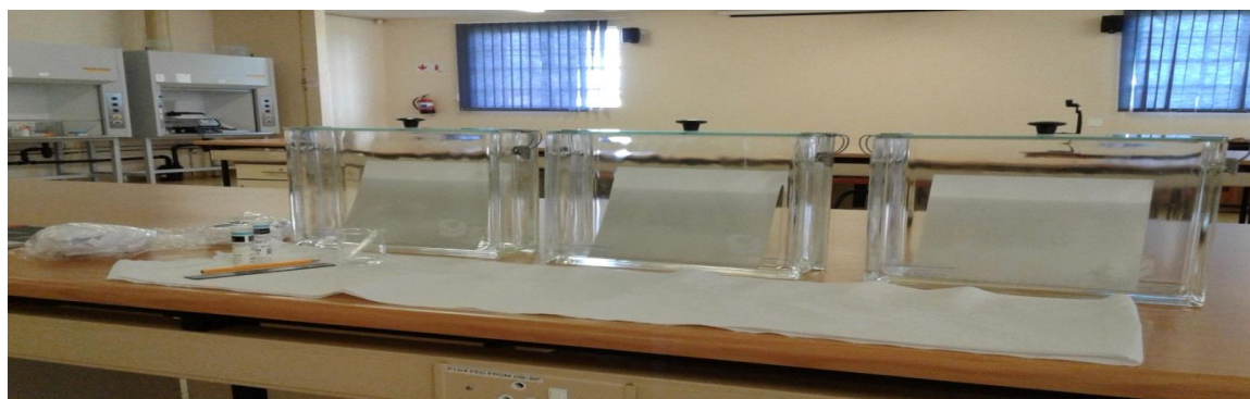
Figure 3.4: Image of standards and samples in a TLC chamber with mobile phases
