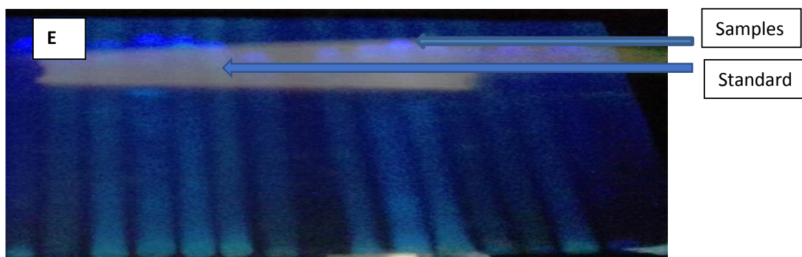
Figure E: TLC plates showing ciprofloxacin under UV light
