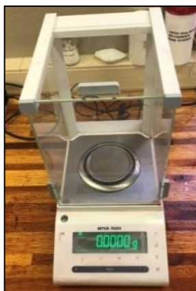
Figure E.6: Mettler Toledo balance used to determine mass loss
