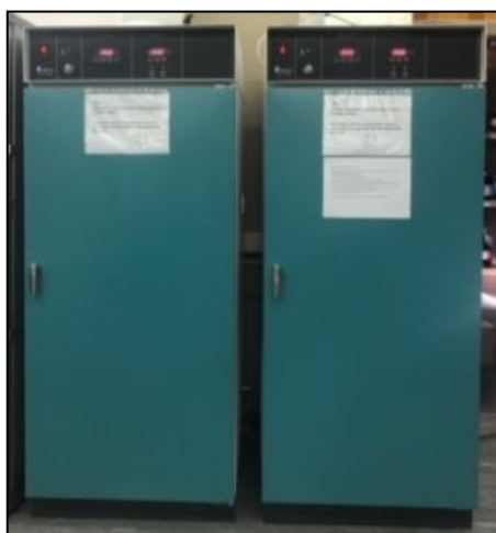
Figure E.1: Labcon® humidity chambers used to perform accelerated stability tests
