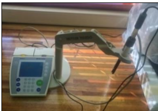
Figure E.3: Mettler Toledo pH meter used to perform pH measurements
