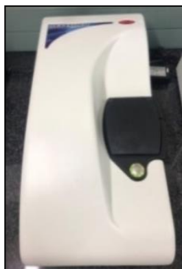
Figure E.5: Malvern zeta-sizer Nano ZS used to measure zeta-potential
