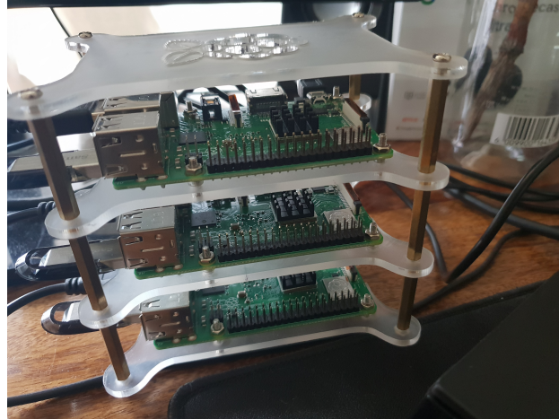
Figure B.1 Improved cooling of Raspberry Pi's using an open airflow case and aluminium heatsinks.
