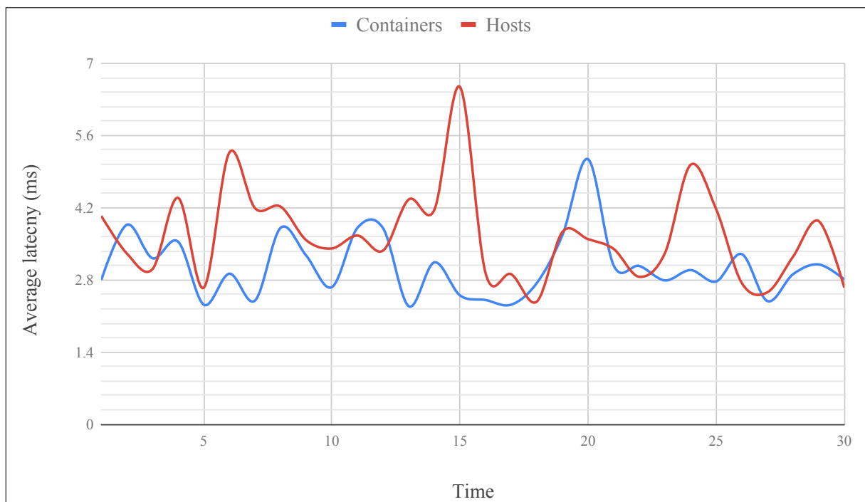
Figure 4.13 Latency comparison between direct networking over 802.11n network and Docker Swarm overlay network.
