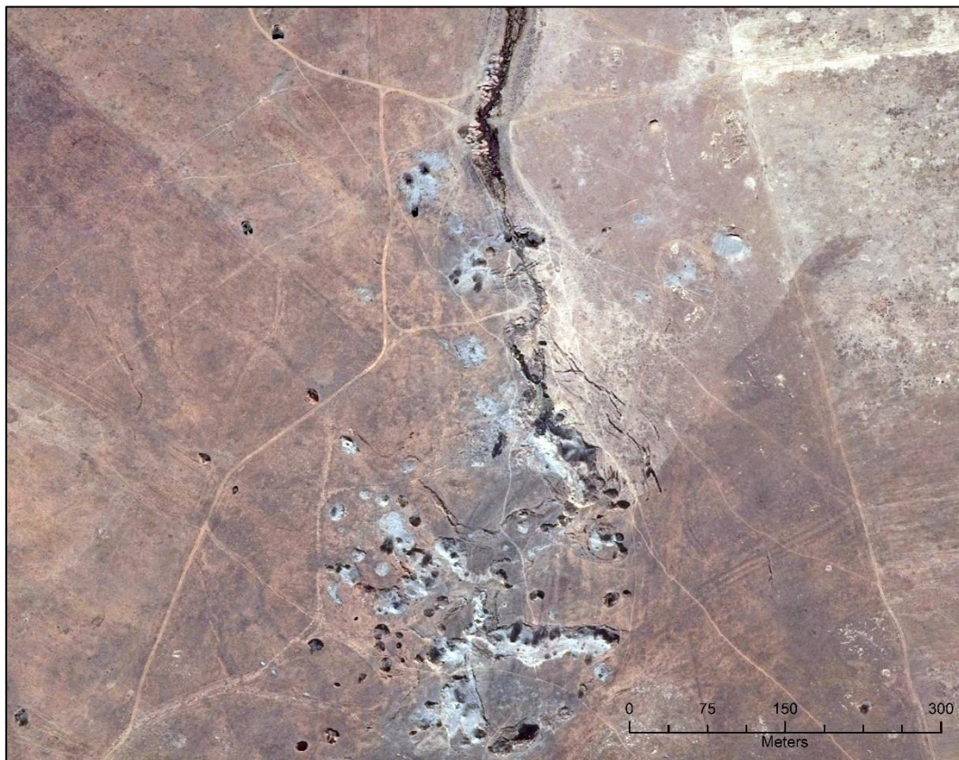
Figure 32: Sinkhole cluster located in the Venterspost Compartment (NGI, 2015).
