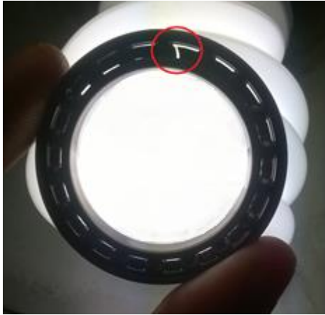
Bearing at suspected failure for multiple 4000 r/min delevitations
