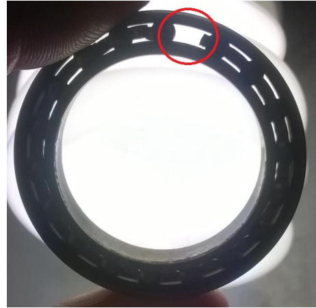
Bearing at suspected failure for random delevation conditions
