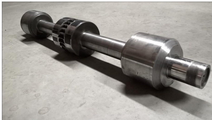
Figure 3-2: Rotor used for experimental delevitation
