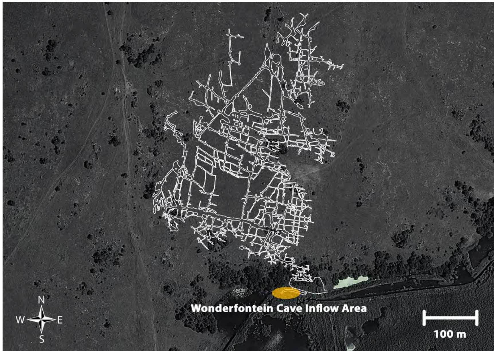
Figure 2.2: A survey map of the Wonderfontein Cave system plotted over a satellite image of the area where it is situated, illustrating the extent of the cave system and associated Wonderfontein Cave inflow area (Photo: Google Earth, available at https://www.google.com/earth ).
