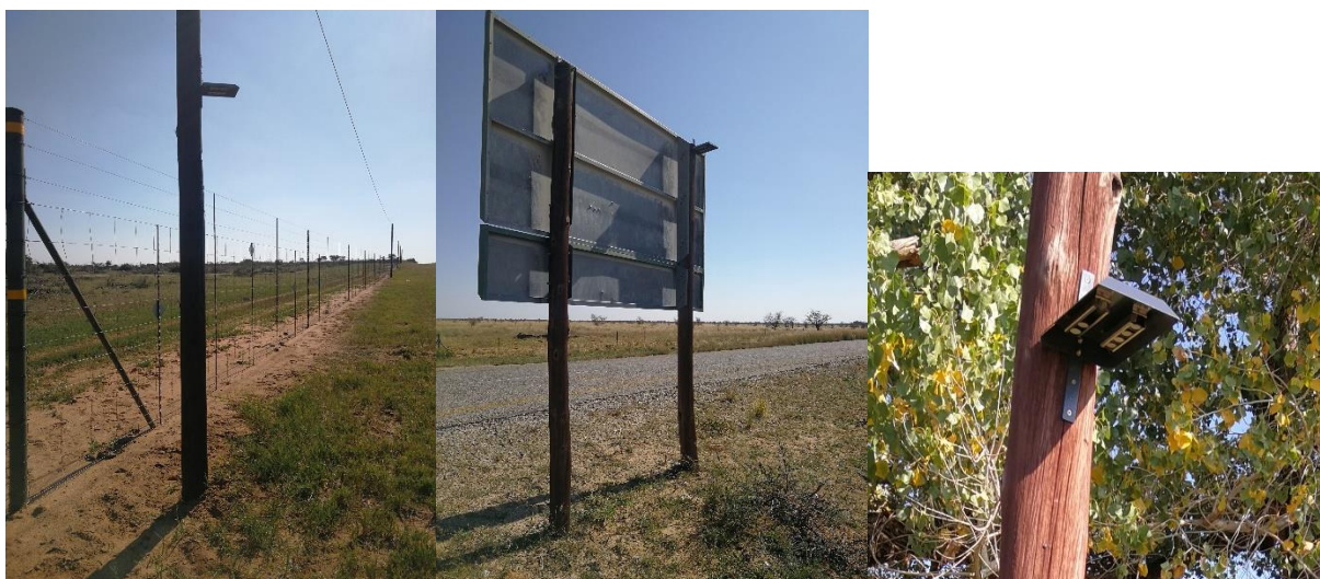
Figure 3.2.3. Examples of sampler hoods used during the intensive campaign, which were attached to telephone/electrical poles, or road signs.
