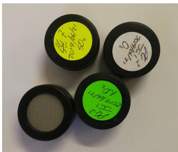
Figure 3.2.1. Photo of assembled passive samplers before being deployed.
