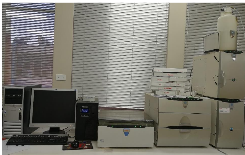
Figure 3.2.4. The Ion Chromatography Dionex ICS 3000 used for determining passive sample concentrations.
