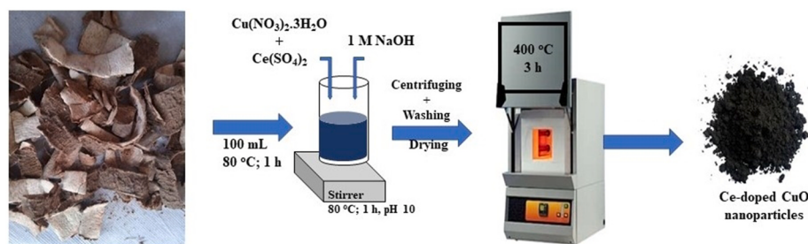
Fig. 1. Schematic for the synthesis of Ce-doped CuO from aqueous extract of yam peel.
